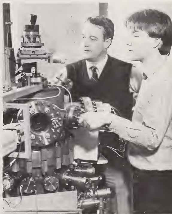
Drs. Ted Madey and Allen Johnson use electron stimulated desorption ion angular distribution to determine how atoms and molecules are bonded to the surface.
