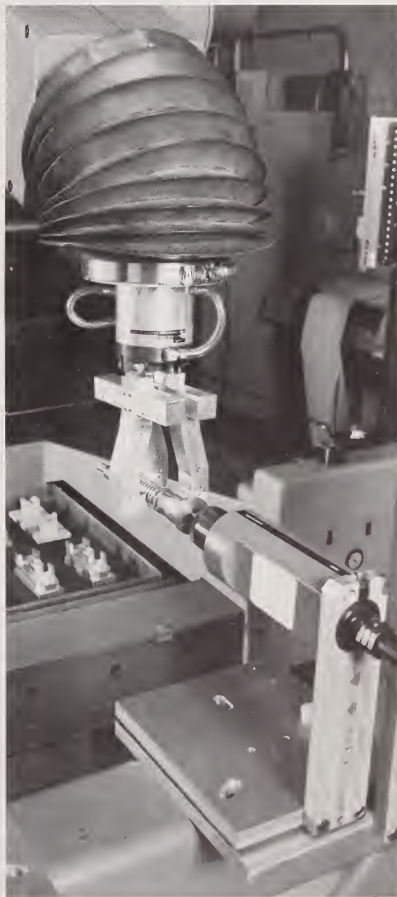
A robot at the AMRF inspection workstation presents a newly machined part to a device that uses optical techniques to measure surface finish.
