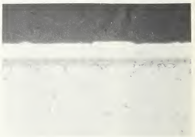
(f) 0.00015-in. nickel under 0.0003-in. gold coating.
