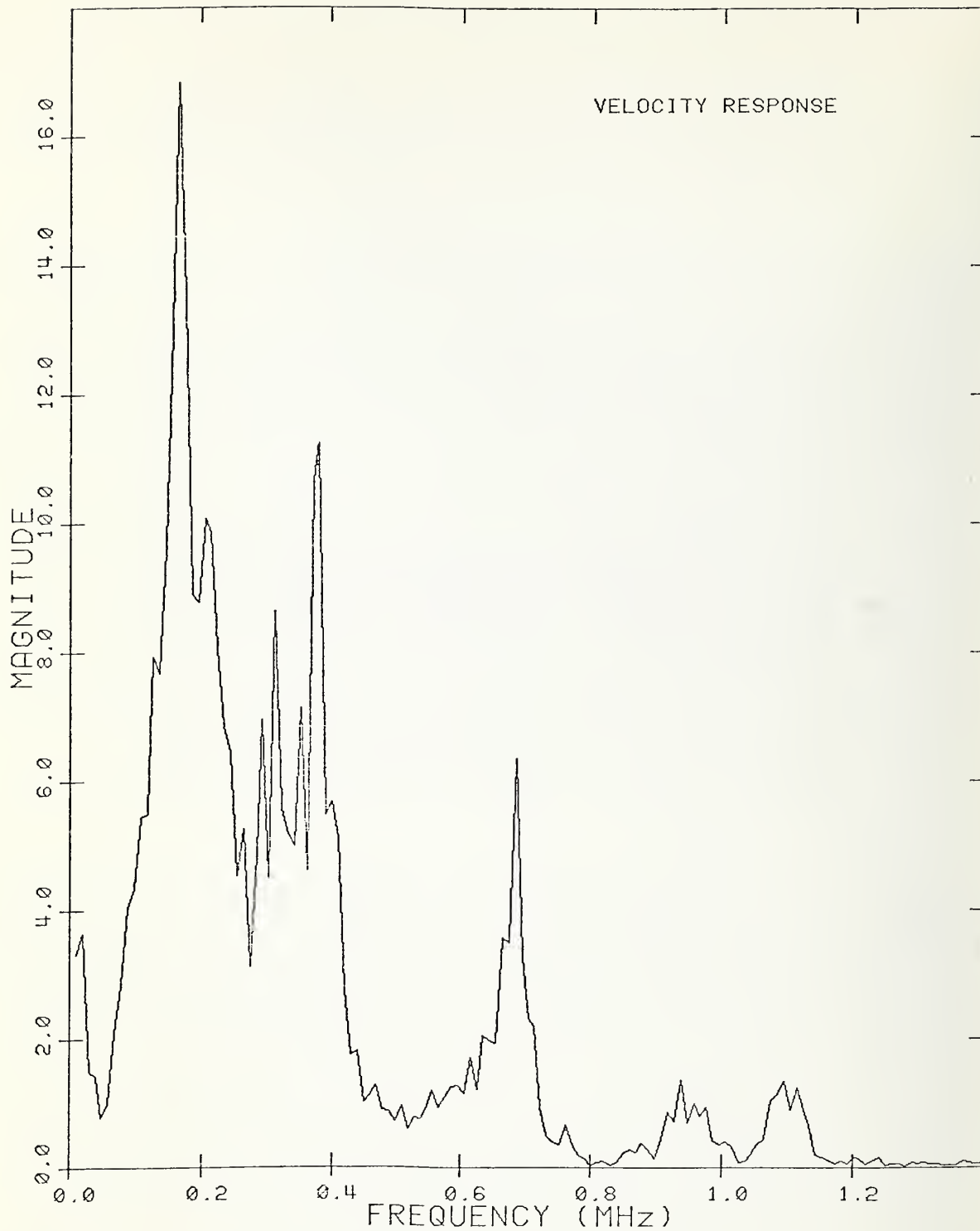
Figure 15. The frequency spectral response of a TO-100 acoustic-emission detector-preamplifier. (The PZT ceramic element used in this test was designed for a 1-MHz peak response.)
