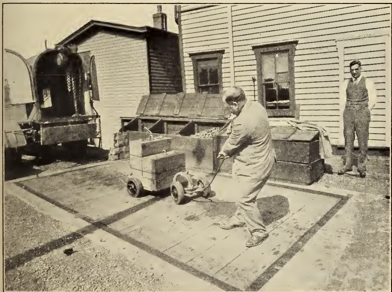
FIG. 3.—"Spot" testing with mobile 3,000-pound testing unit—New Jersey equipment
