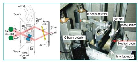
Fig. 1. A picture of the setup is shown on the right and a schematic plan view is shown on the left.
