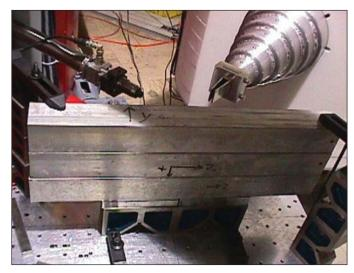
Fig. 1. The measurement configuration on the BT-8 instrument at the NCNR for residual stress determinations on three 2024 AI bars. Neutrons issuing from the collimated beam tube on the left are collected from the sample volume by the detector on the right. The sample is scanned by moving the mounting table.
