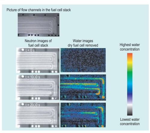
Fig. 3. A fuel cell: gas distribution channels shown disassembled on top. When assembled, images of the operating cell were taken every second for 2000 seconds. The water build-up in both the gas diffusion media and the flow channels is most clearly visible in the colorized images in which the underlying dry fuel cell has been computationally removed.
