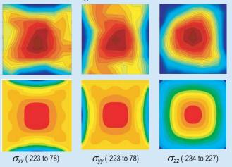
Stresses (in MPa) calculated by finite-element method: min (blue) to max (red)
