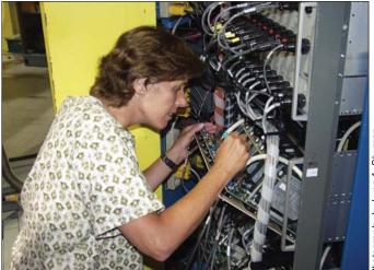
Fig. 3. Doris Kendig (NCNR) adjusts motor drivers on the new motor control system.
