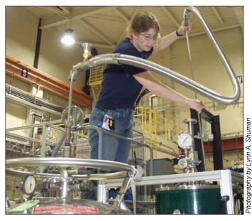
Fig. 4. Rachel Anderman (NCNR) fills the new 9T horizontal field superconducting magnet with helium.
