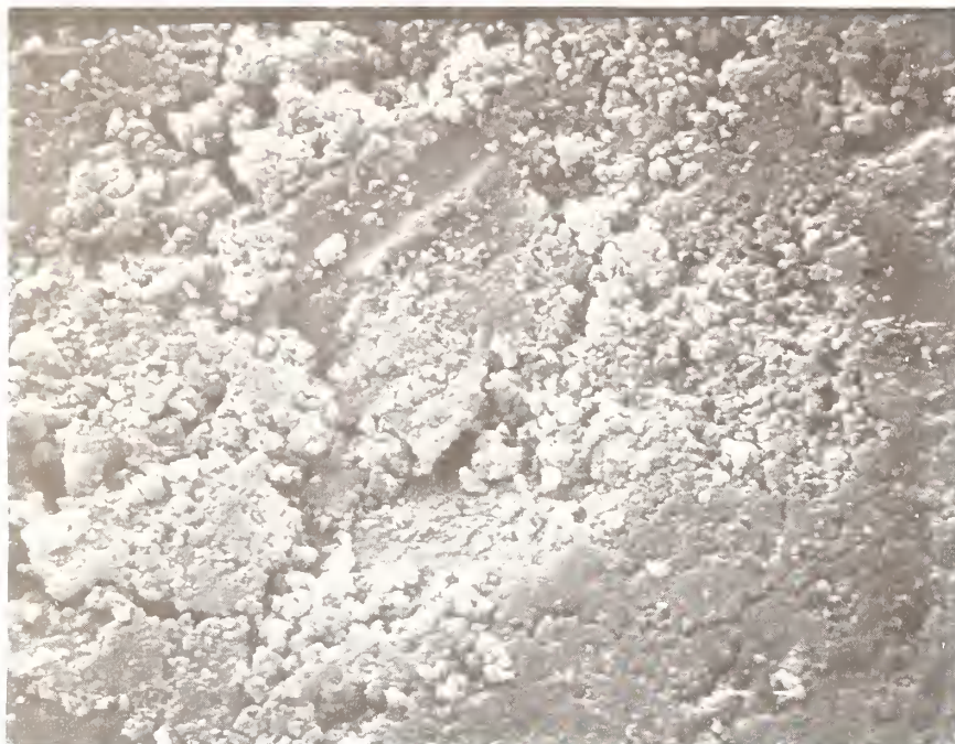
Figure 36. SEM Photomicrograph of Upper Specimen Wear Track Water-Lubricated Run 2748R - 5000X
