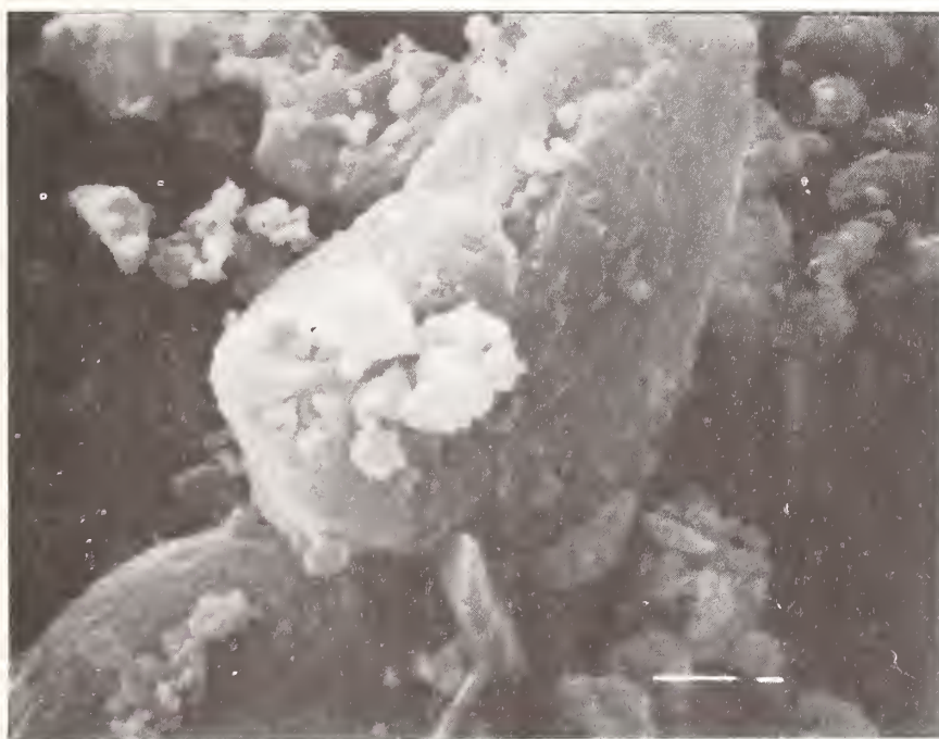
Figure 64. 10,000X Secondary Emission SEM Photograph of Powder AL1
