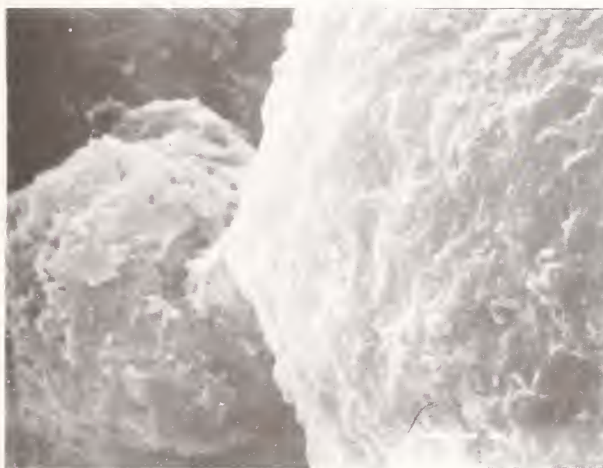
Figure 68. 10,000X Secondary Emission SEM Photograph of Powder AL3
