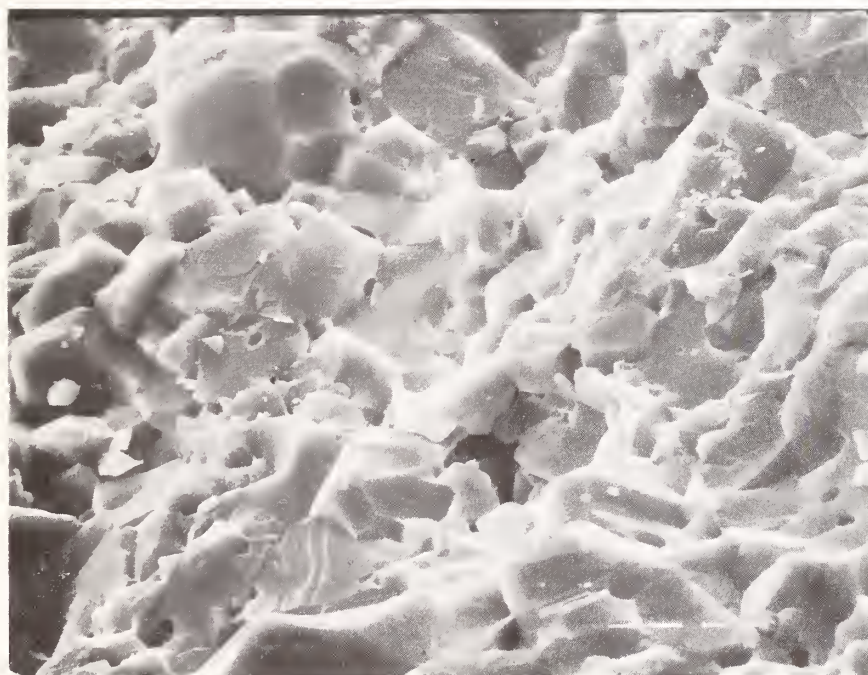
Figure 6. SEM Photomicrograph of Fracture Surface of Cer 005 Alumina - 1000X
