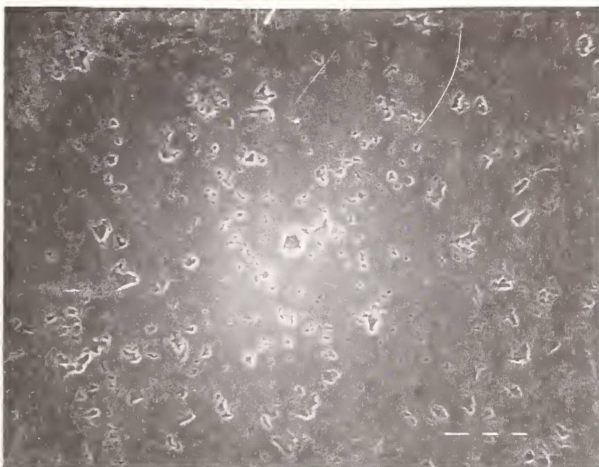
Figure 11. SEM Photomicrograph of Polished Surface of Cer 006 Alumina - 500X
