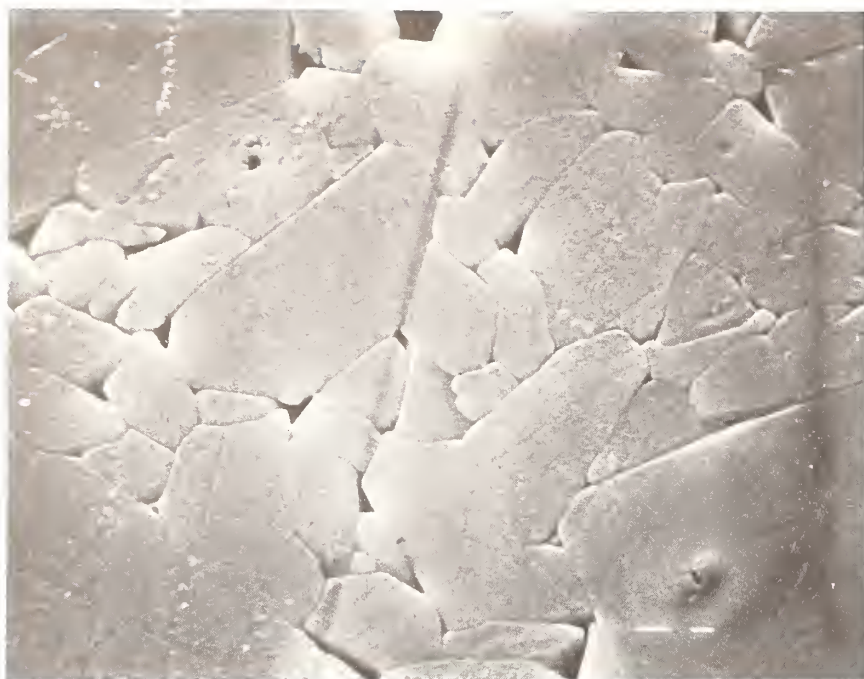
Figure 13. SEM Photomicrograph of Polished/Etched Surface of Cer 004 Alumina - 5000X
