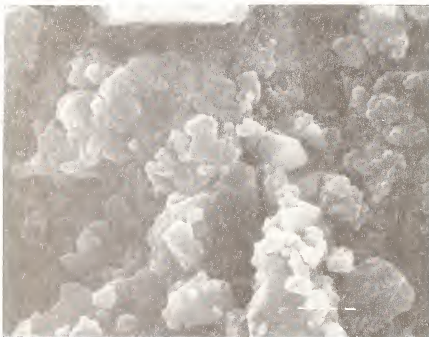
Figure 43. SEM Analysis of Wear Debris from Paraffin Oil Lubricated Wear Test - 10,000X
