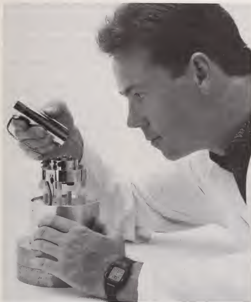
Engineer Paul Rice positions the piezoelectric scanner of a scanning tunneling microscope designed to study magnetic features in materials with submicron resolution.
