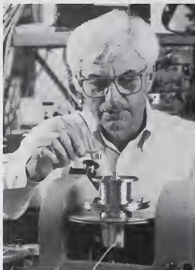
Chemist Lloyd Weber measures chemical and physical properties of alternate refrigerants. The goal is to help industry find effective replacements for chlorofluorocarbons or CFCs, which break down the Earth's ozone layer.
