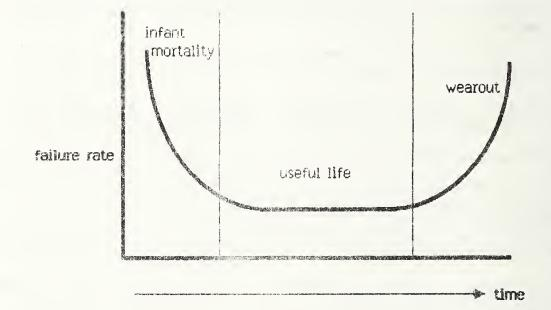
As the system gets older, more failures occur due to wear-out of the components. The time to repair increases because of the difficulty in obtaining replacement parts and knowledgable repair personnel.
