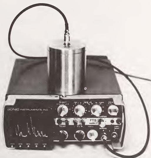
Figure 6b. Registration of the Specific Ultrasonic Pattern of Each Can
