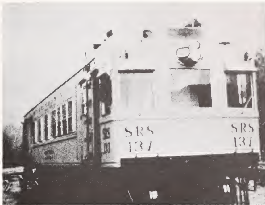
(A) RAIL BOUND DETECTOR CAR OWNED AND OPERATED BY SPERRY RAIL SERVICE
