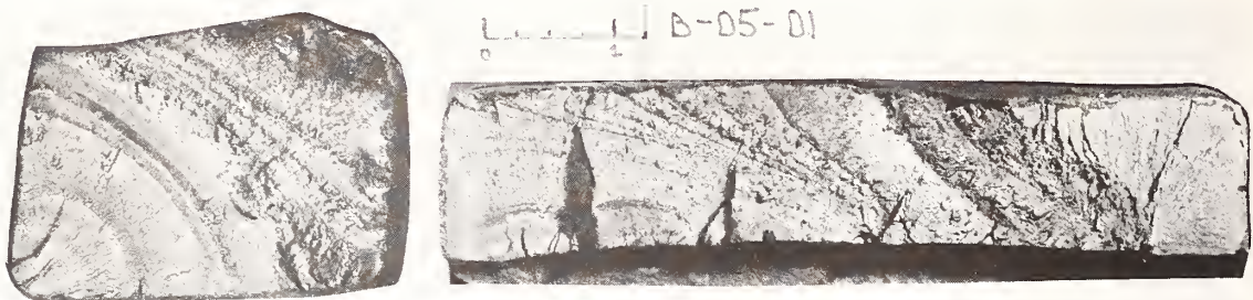
Figure 3: Large fatigue cracks in failed coupler (A-01) and yoke (B-05).
