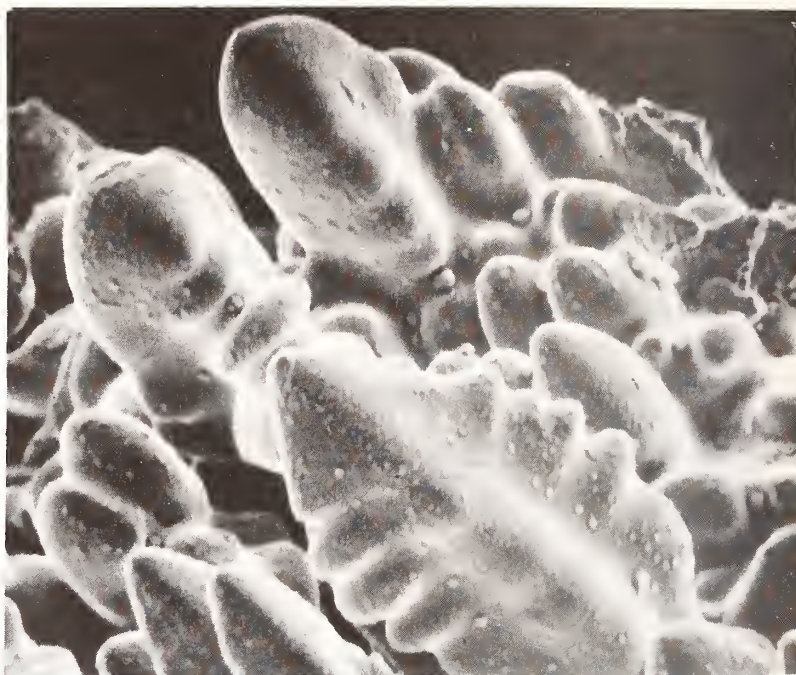
Figure 9: A three dimensional dendrites pattern, in a shrinkage cavity, C(N&T) grade, B-05 yoke (X150).
