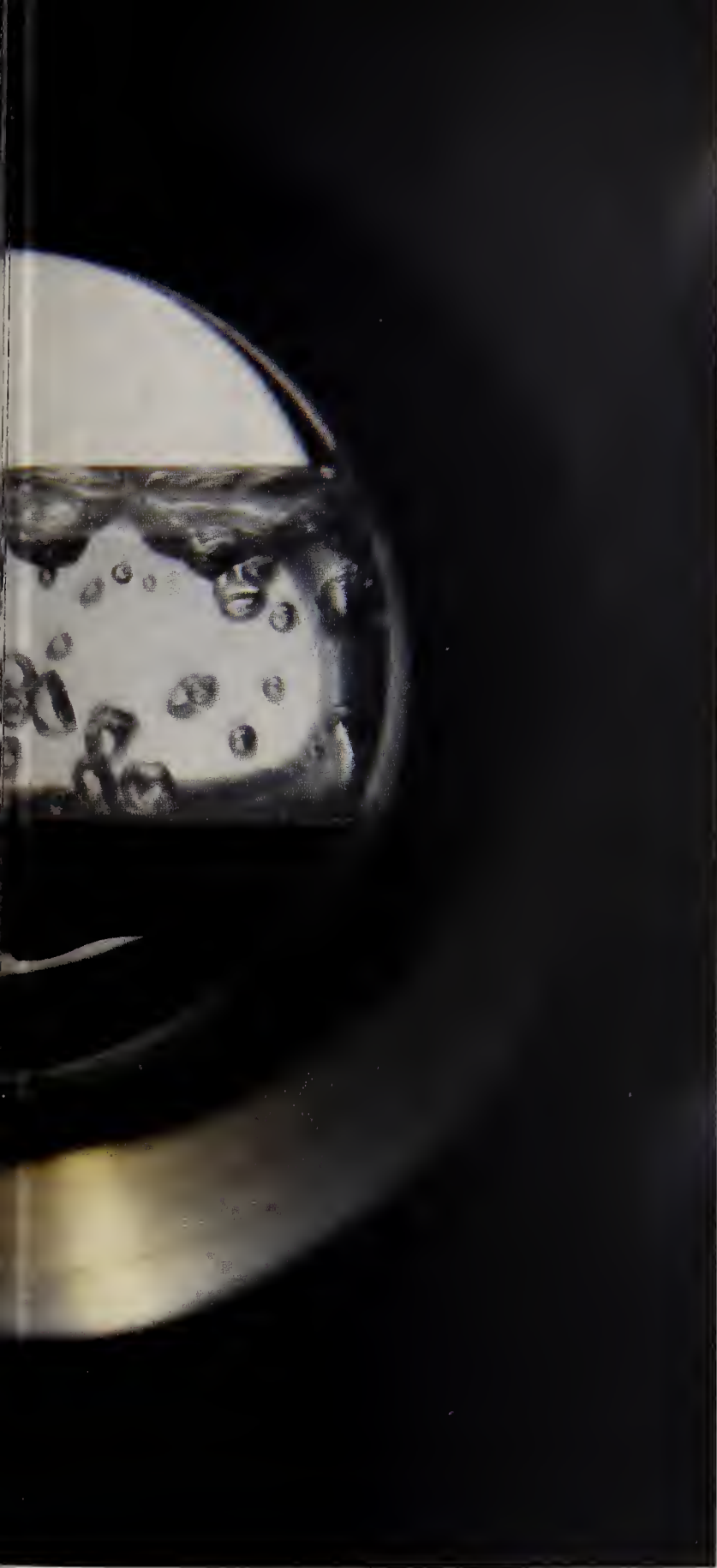
Above. NIST researchers study the boiling properties of new environmentally compatible refrigerants in order to help industry improve the effectiveness of building air-conditioning systems.
