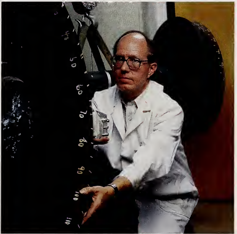
Top. Technician Max Peltz examines cracks on a precast concrete beam being tested for strength and ductility at the NIST tri-directional test facility.
