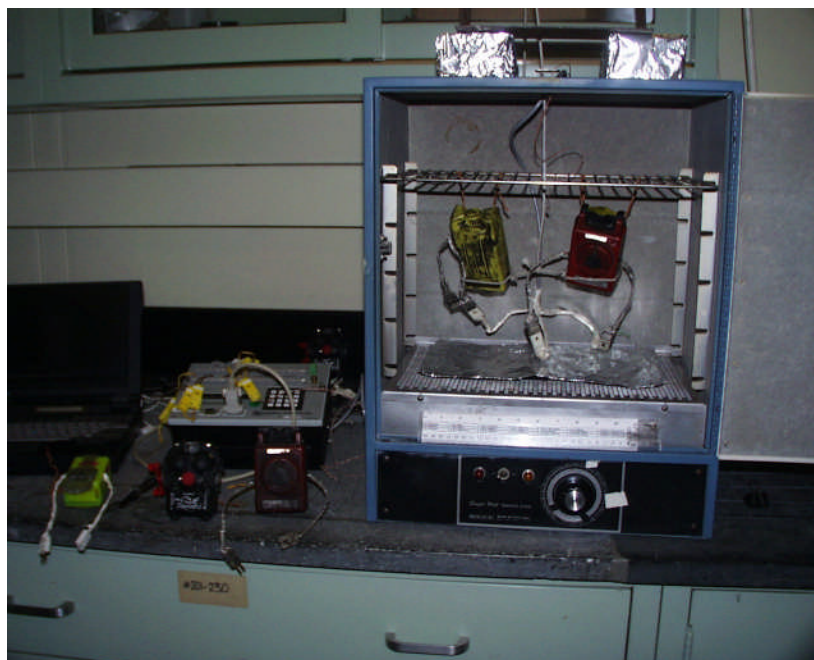
Figure 4. Photograph of static oven apparatus.
