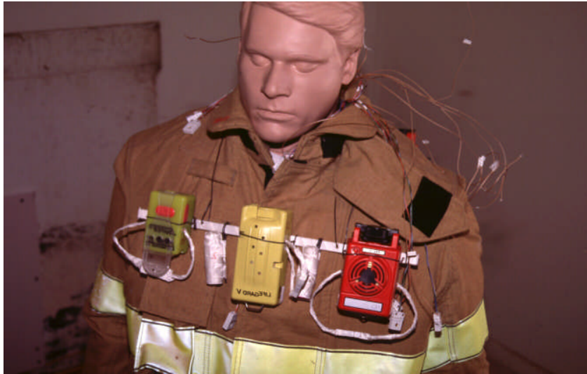
Figure 9. PASS devices positioned on front of mannequin.
