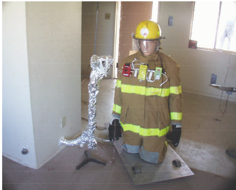
Figure 7. Instrumented mannequin for full-scale field experiments.
