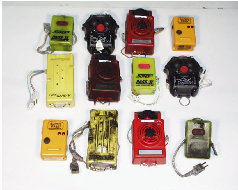
Figure 1. Personal Alert Safety System (PASS) devices from various manufacturers.
