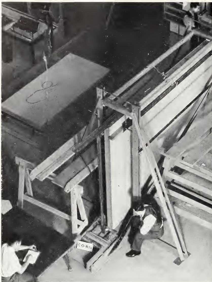
FIGURE 44.— Partition specimen CO-R1a under racking load.
