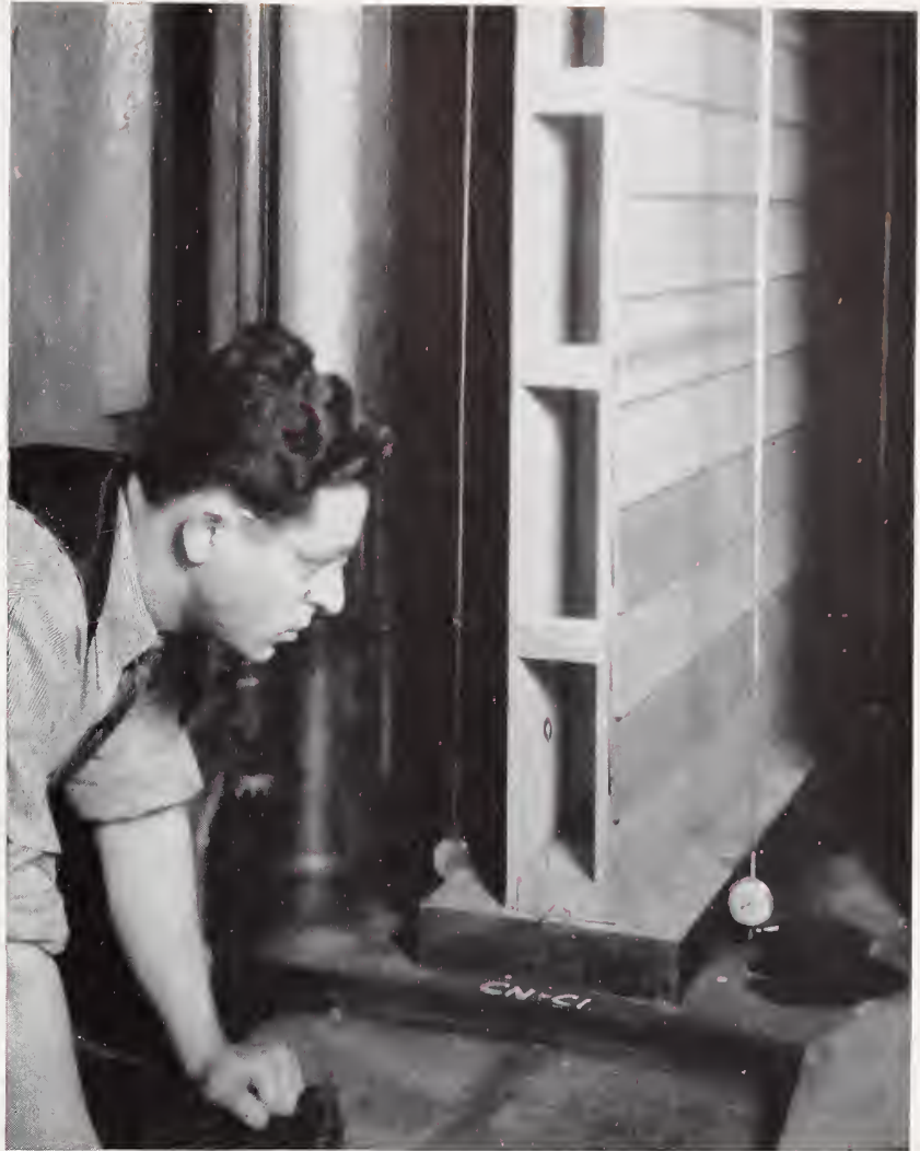
FIGURE 27.—Wall specimen CN-C1 under compressive load.
