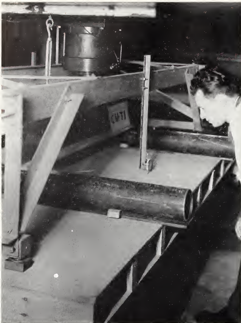
FIGURE 13.—Wall specimen CM-T1 under transverse load.
