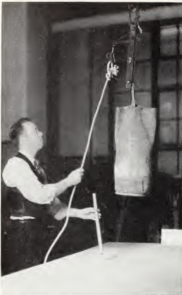
FIGURE 18.—Wall specimen CM-14a during the impact test.
