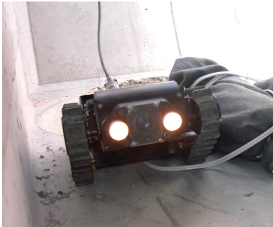
Figure 5a. Shape-shifting robot in lower configuration.
