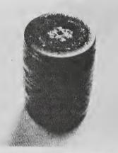
Moisture in the lubricant can cause rusting on a roller end—or on the roller surface if it is inactive.
