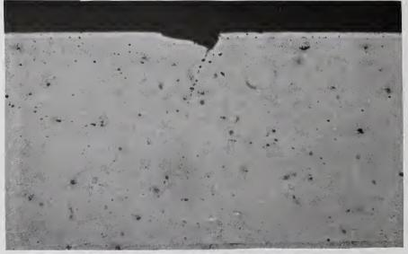
FIG. 7 Crack Propagation from an Indentation with 40 Micron Filtration (× 500).
