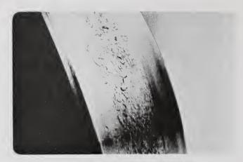
Smearing is another result of inadequate lubrication, as two surfaces adhere, and metal from one surface is actually welded to the other.
