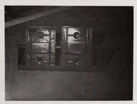
Figure 5. A corroded and a new battery tray.
