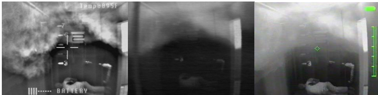
Figure 1. View of a corridor with a heated mannequin on the floor, and a temperature target and reflective strips on the back wall. Hot, smoke-laden gases are entering the corridor from an adjacent room on the right. The three TICs are viewing an identical scene at the same moment.
