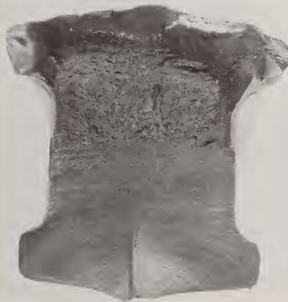
FIGURE 22. Fatigue fracture in a truck axle. The vertical dimension of the axle is 7.5 cm.
