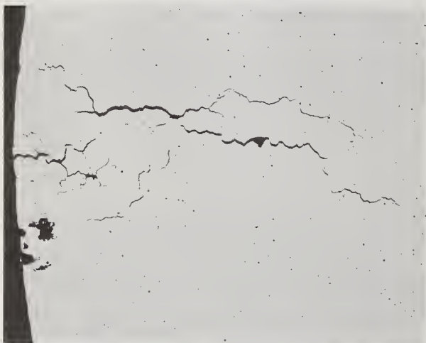
FIGURE 17. Section of the collar of figure 16 showing cracks remote from the fracture. \times 75 .
