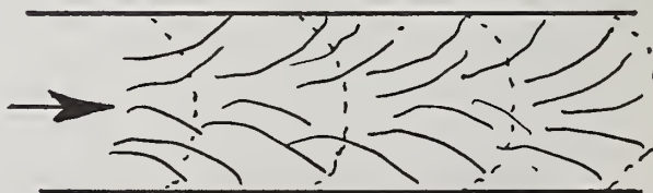
FIGURE 5. Sketch showing the development of fracture markings (solid lines) perpendicular to the moving crack front (dotted lines).
