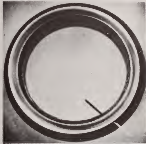
Fig. 2 Tungsten carbide mechanical seal face showing symmetrical surface polishing characteristic of mild hydraulic or thermal distortion
