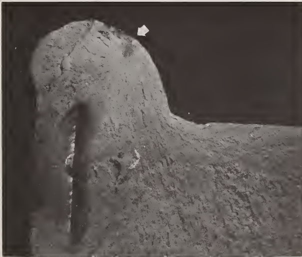
FIGURE 6. Area near the origin of the fracture in a B-52 bulkhead. X4.
