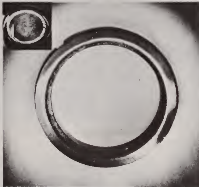
Fig. 3 Tungsten carbide mechanical seal face showing localised polishing due to lack of flatness, this seal leaked badly The inset illustrates a typical non flat seal face viewed in sodium light using an optical flat to give contour lines at 11 micro inch increments of height
