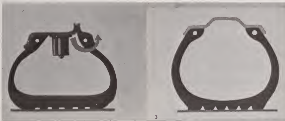
FIGURE 14. Comparison between standard tyre and Dunlop Safety Tyre—Leeds Industrial Unit of Tribology.
