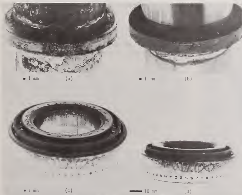
FIGURE 11. Fretting damage of fitted surfaces. (a) and (b) are fretted shafts from heavily loaded tests.
