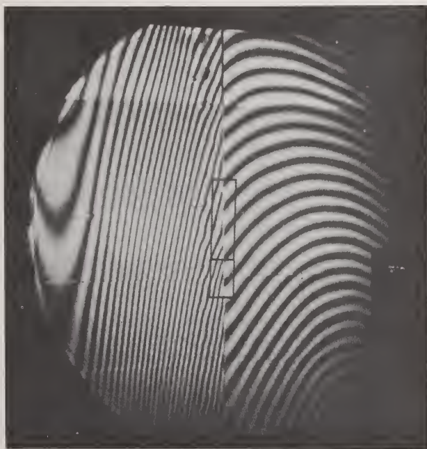
FIGURE 18. Demonstration that surface paint does not degrade the quality of the interferometric fringe pattern. Original flaw still evidenced by discontinuity in fringe pattern in boxed area.
