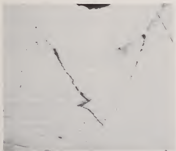
FIGURE 5. Mid-thickness crack configuration in U-notched AISI 4340 specimen loaded close to maximum load [31]. Steel tempered to 178 ksi ultimate tensile strength. \times 90 .
