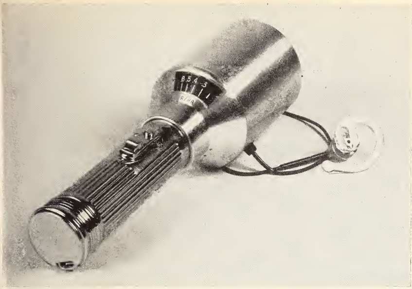
Portable radioactivity survey instrument developed by NBS for gamma radiation (p. 72). The device is extremely rugged and compact.
