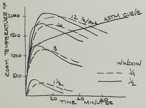
In general, the tests with 1/4 window area seemed to provide the most severe exposure although peak temperatures were somewhat less.
