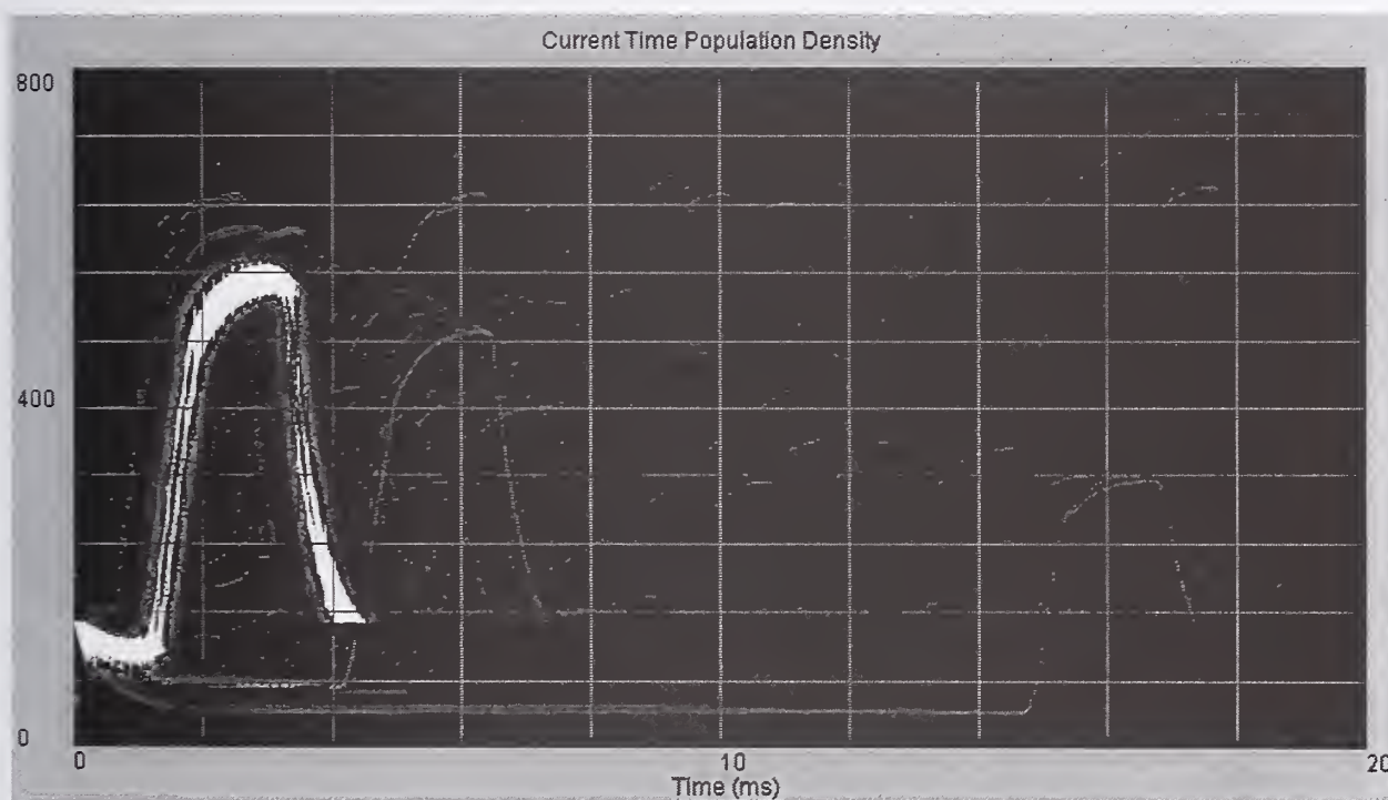
Figure 10: Pulsed spray transfer arc voltage vs. time density plot from PowerWave 455, L-50 electrode, and 90% Ar+10% CO 2
