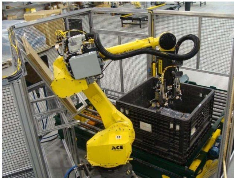
Figure 9 – Vision system being used to guide the robot to load a box with parts ( www.fanucrobotics.com ). [copyright photo-use permission granted by Fanuc Robots]
