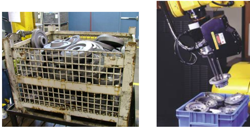
Figure 12 – (left) bin of parts ( www.tec-automation.com/.../random-bin-picking/ ), (right) robot picking parts from a bin ( www.adaptivesystems-usa.com/integ_assembly.asp ) [copyright photo-use permission granted by Fanuc Robots]
