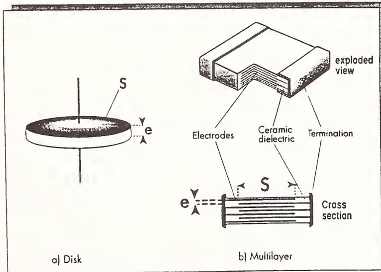
Figure 2: Ceramic Capacitors
