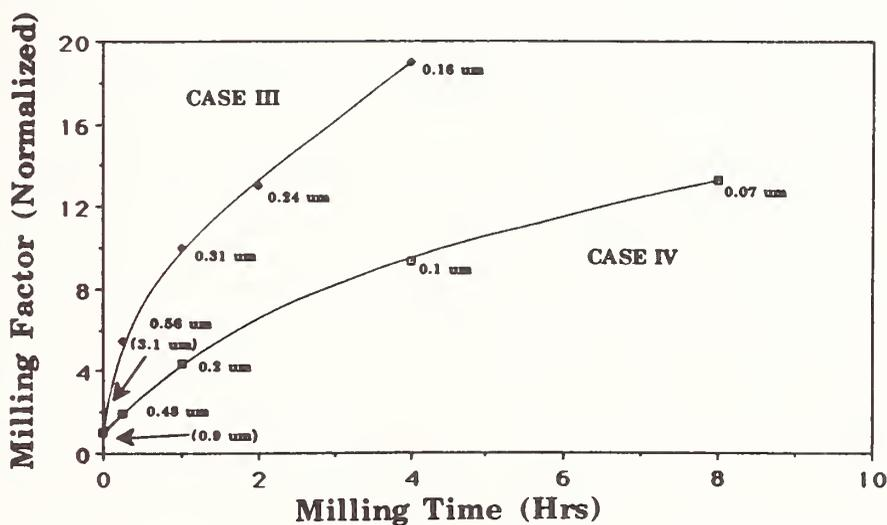
Figure 4. Milling factor (normalized) for reactively calcined PZT (Cases III (3.1  $\mu\text{m}$ ) and IV (0.9  $\mu\text{m}$ )) as a function of milling (attrition) time.
