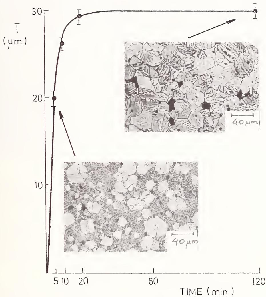
Fig. 1: Average intercept length vs. sintering time and corresponding microstructures for BaTiO<sub>3</sub> - TiO<sub>2</sub> excess ceramics, sintered at 1350°C
