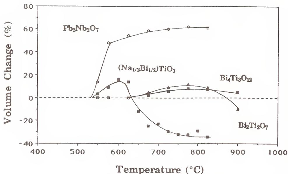
Figure 5. Volumetric expansion-shrinkage characteristics of  $\text{Pb}_2\text{Nb}_2\text{O}_7$ ,  $\text{Bi}_2\text{Ti}_2\text{O}_7$  (pyrochlore),  $\text{Na}_{0.5}\text{Bi}_{0.5}\text{TiO}_3$  (perovskite) and  $\text{Bi}_4\text{Ti}_3\text{O}_{12}$  (larger structure).
