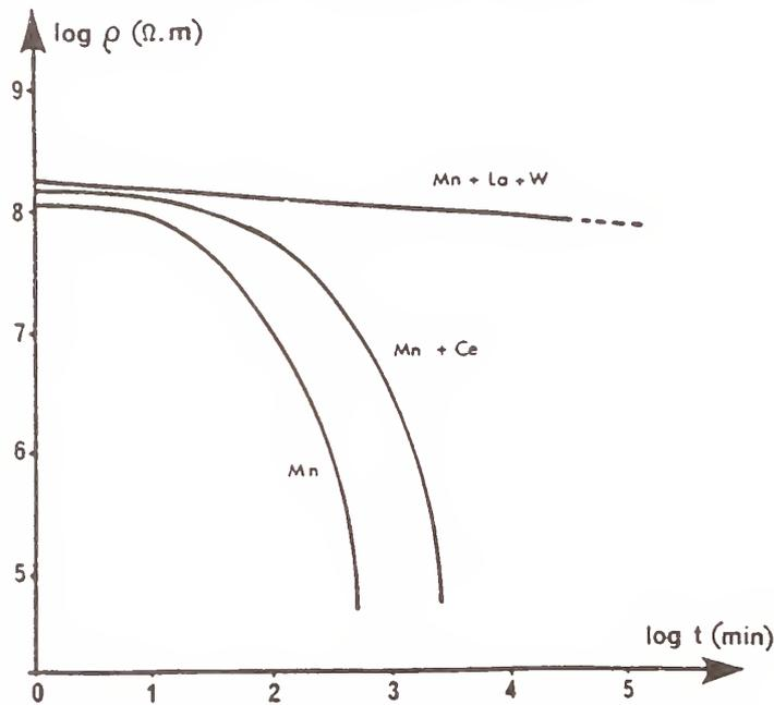
Figure 6: Resistivity of BaTiO<sub>3</sub> based Z5U material as a function of various doping during life test (1.7V/μm and 280°C) [3].
