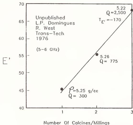
Fig. 17. "Processing" versus  $E'$  for " $\text{La}_{2/3}\text{TiO}_3$ " composition.
