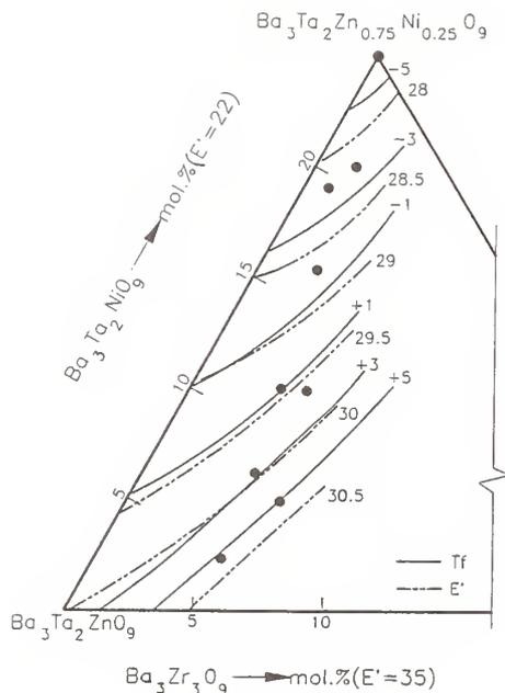
Fig. 16.  $T_f$  and  $E'$  isopleths (approximate) for ordered perovskite ceramics in the system  $\text{Ba}_3\text{Ta}_2\text{ZnO}_9$ - $\text{Ba}_3\text{Ta}_2\text{NiO}_9$ - $\text{Ba}_3\text{Zr}_3\text{O}_9$ . Ten Kg batches were made; fired densities are  $>7.70$  g/cc.
