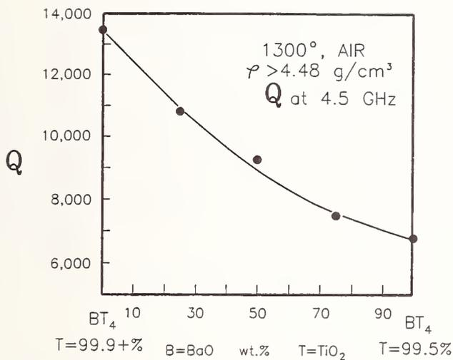
Fig. 1. Q of BaTi<sub>4</sub>O<sub>9</sub> ceramics versus TiO<sub>2</sub> raw material content. Temperature in °C.
