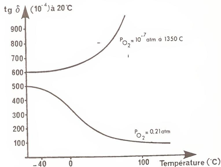
Figure 3: Influence of the oxygen partial pressure during the sintering of a Z5U material with general formula  $Ba_{1-x}Ca_xTi_{1-y}Zr_yO_3$  [3].
