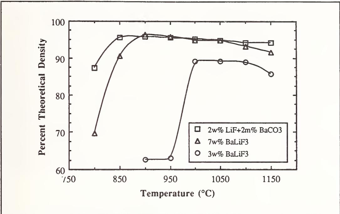
Figure 1: Densification behavior of BaTiO<sub>3</sub> sintered with LiF and BaLiF<sub>3</sub>
