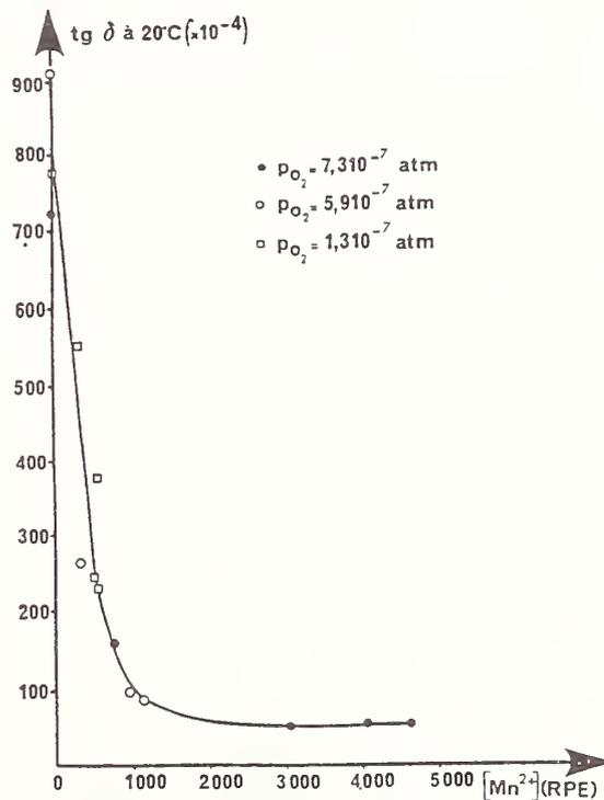
Figure 5: Dielectric losses at Room Temperature as a function of Mn(+II) concentration in a BaTiO<sub>3</sub> based Z5U material [2].
