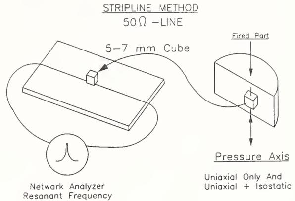
Fig. 13. Method to detect  $E'$  anisotropy in ceramics of Fig. 12.
