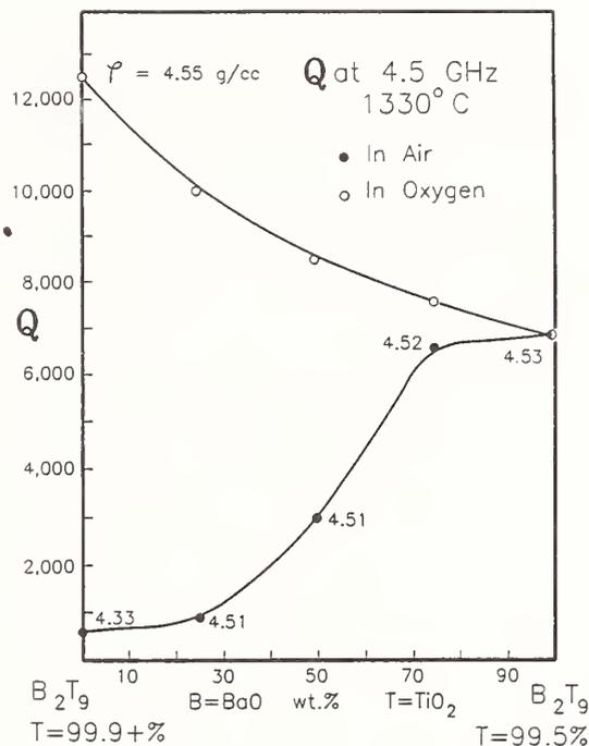
Fig. 2. Q of Ba<sub>2</sub>Ti<sub>9</sub>O<sub>20</sub> ceramics versus TiO<sub>2</sub> raw material content and processing in O<sub>2</sub>/air. 99.9+ %TiO<sub>2</sub> = HP and 99.5%TiO<sub>2</sub> = LP in text.
