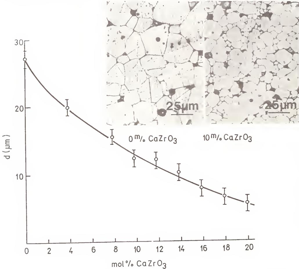
Fig. 6: Average grain size vs. composition in BaTiO<sub>3</sub> - 2 mol % TiO<sub>2</sub>-CaZrO<sub>3</sub> ceramics sintered 1 hour at 1360<sup>0</sup>C
