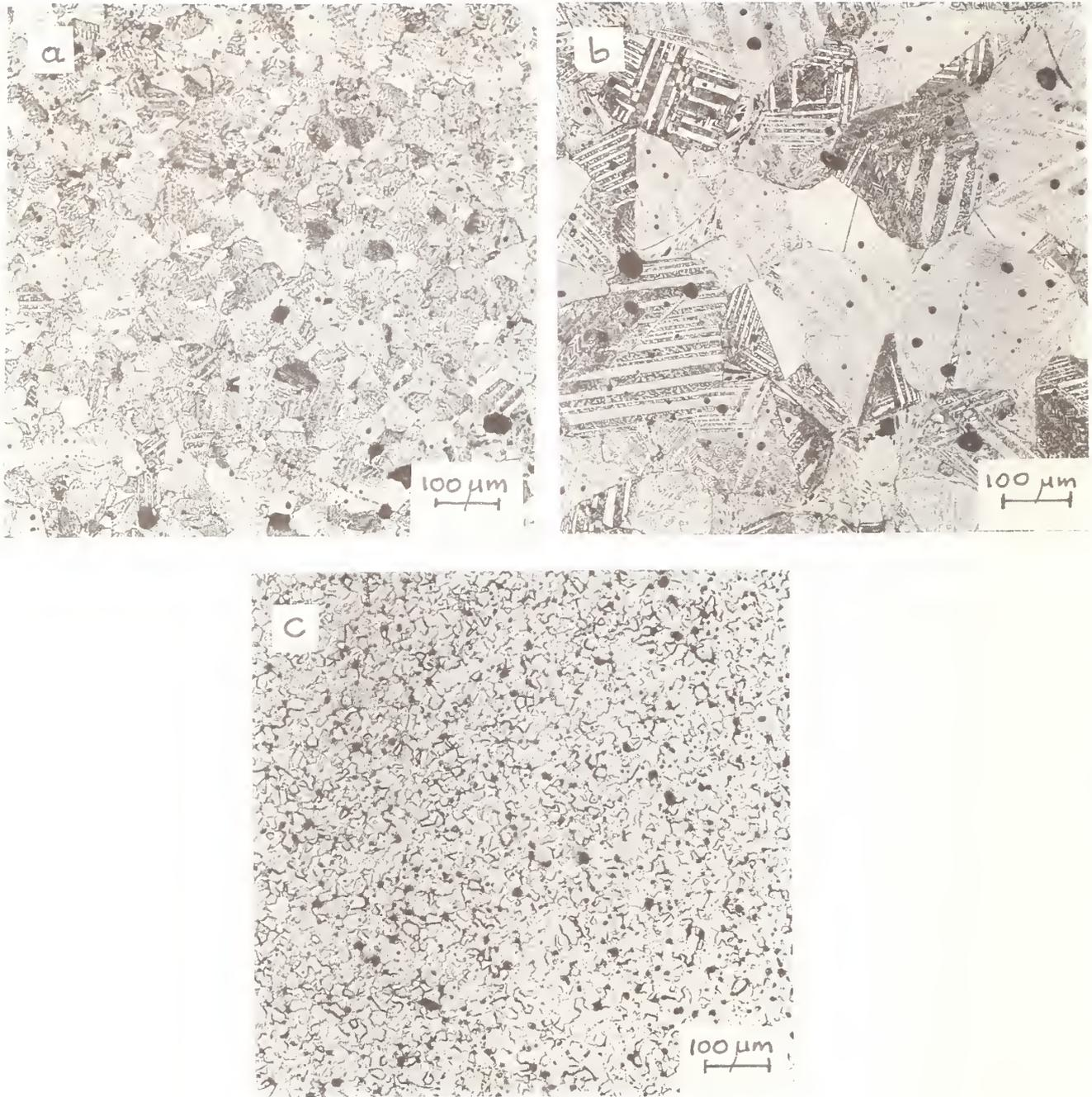
Fig. 2: Microstructures of BaTiO<sub>3</sub> ceramics after heat treatment 24 hours at 1350°C (a) BaTiO<sub>3</sub>-2 mol % Ba<sub>6</sub>Ti<sub>17</sub>O<sub>40</sub>, (b) BaTiO<sub>3</sub> - 2 mol % Ba<sub>6</sub>Ti<sub>17</sub>O<sub>40</sub> - 8 mol % CaTiO<sub>3</sub>, (c) BaTiO<sub>3</sub> - 2 mol % Ba<sub>6</sub>Ti<sub>17</sub>O<sub>40</sub> - 8 mol % SrTiO<sub>3</sub>
