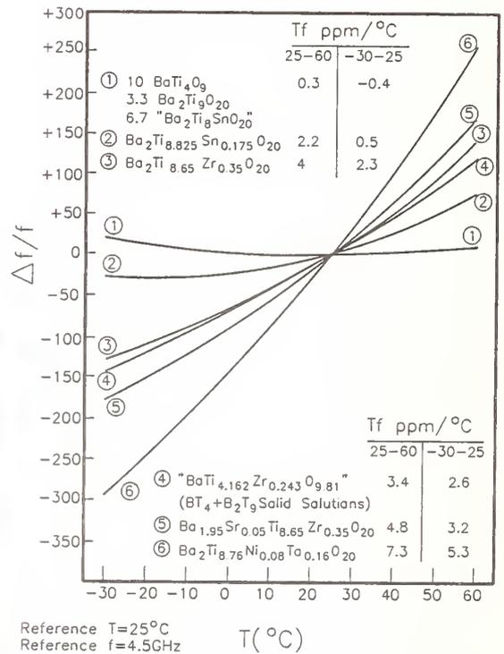
Fig. 8.  $\Delta f/f$  versus temperature ( $T_f = \Delta f/f\Delta T$ ) for ceramics based on  $Ba_2Ti_9O_{20}$  that contains various cation substitutions; 25-60, -30-25 in  $^\circ\text{C}$ .
