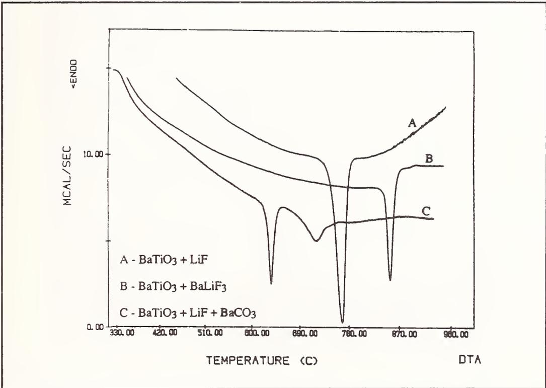
Figure 2: DTA results for mixtures of LiF and BaLiF<sub>3</sub> with BaTiO<sub>3</sub>.
