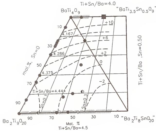
Fig. 6.  $T_f$  isopleths (approximate) for the system  $BaTi_4O_9$ - $Ba_2Ti_9O_{20}$  and  $SnO_2$ -containing solid solutions (1330-1350°C,  $O_2$ ). Hatching depicts approximate limits of solid solubility after (1) and this work (■, not single phase). Open circles are after (5).
