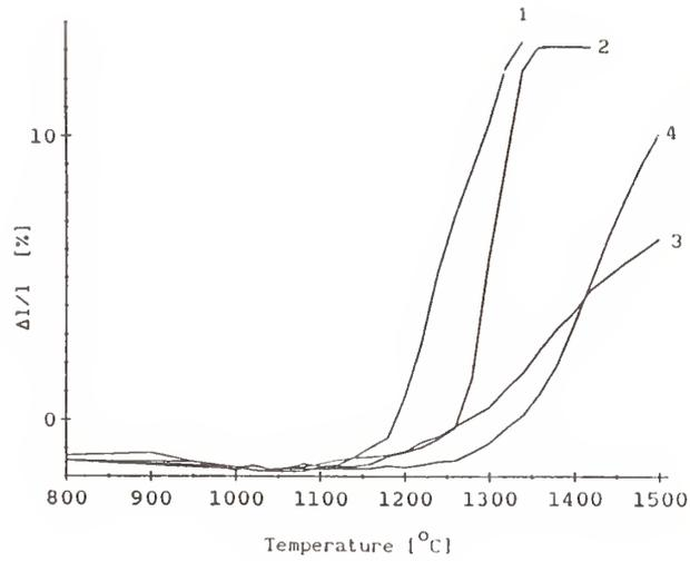
Fig. 5: Dilatometric curves for (1) BaTiO<sub>3</sub> - 2 mol % TiO<sub>2</sub> (2) BaTiO<sub>3</sub> - 2 mol % TiO<sub>2</sub> - 8 mol % CaZrO<sub>3</sub> (3) BaTiO<sub>3</sub> - 8 mol % CaZrO<sub>3</sub> (4) CaZrO<sub>3</sub>. Heating rates 10<sup>0</sup>C/min
