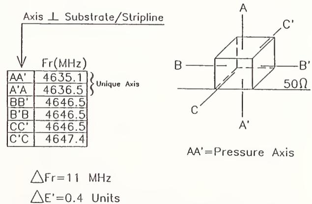
Fig. 14. Methodology and example measurements to determine  $E'$  anisotropy by the "cube technique", Fig. 13.
