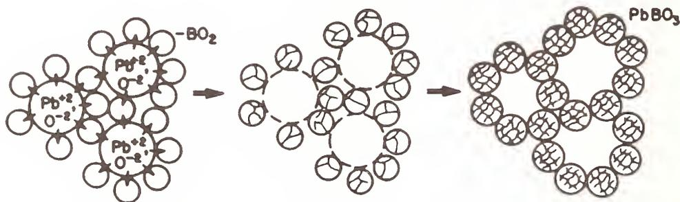
Figure 1. Schematic representation of the perovskite  $\text{PbBO}_3$  formation and associated morphological changes.<sup>(3)</sup>
