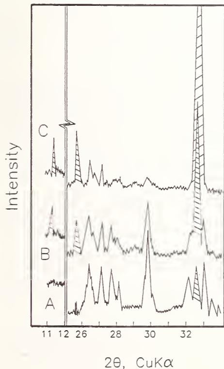
Fig. 18. XRD tracings for ceramics in Fig. 17 (A,B,C correspond to  $E' = 45, 55, 68$ , respectively). A =  $\text{LT}_2 + \text{L}_2\text{T}_9 +$  trace ordered perovskite (P, shaded); B =  $\text{LT}_2 + \text{L}_2\text{T}_9 + \text{P}$ ; C =  $\text{L}_2\text{T}_9 + \text{P}$  (trace  $\text{LT}_2$ ).  $\text{LT}_2 = \text{La}_2\text{Ti}_2\text{O}_7$ ;  $\text{L}_2\text{T}_9 = \text{La}_4\text{Ti}_9\text{O}_{24}$ .
