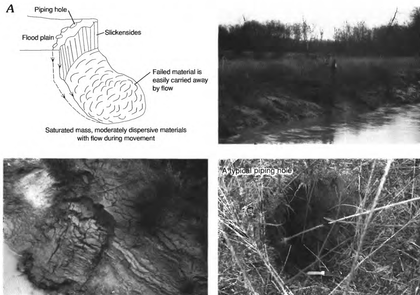
FIGURE 42.—(A) Saturated and (B,C) nonsaturated deep-seated rotational failures.
