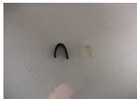
Programming (Deformation), T > T_g
