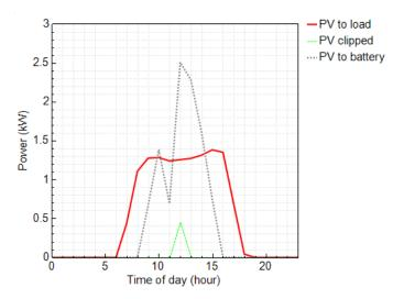
Fig. 5. Operation with a AC-connected battery on March 24
