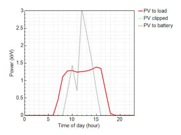
Fig. 4. Operation with a DC-connected battery on March 24
