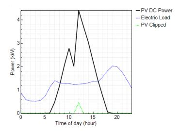
Fig. 3. The site electric load and PV production on March 24
