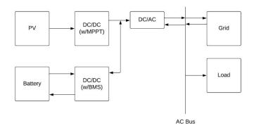
Fig. 1. PV plus DC-connected battery storage system diagram.
