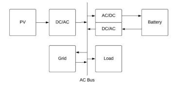
Fig. 2. PV plus AC-connected battery storage system diagram.
