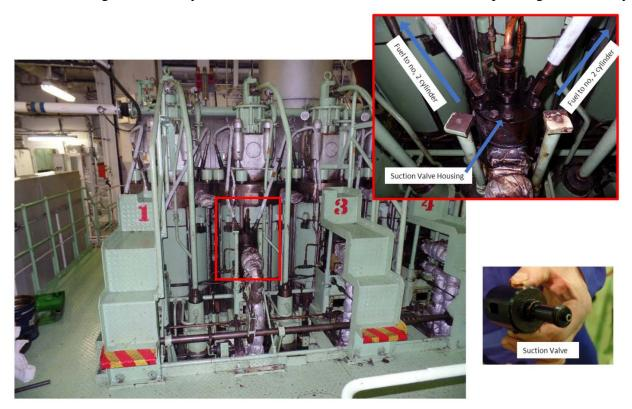
Clockwise from left: cylinder nos. 1 through 4 of the direct-drive diesel engine on *Mia S*; fuel pump for no. 2 cylinder; and non-return/suction valve for no. 2 cylinder fuel pump. (Photos by Coast Guard)
