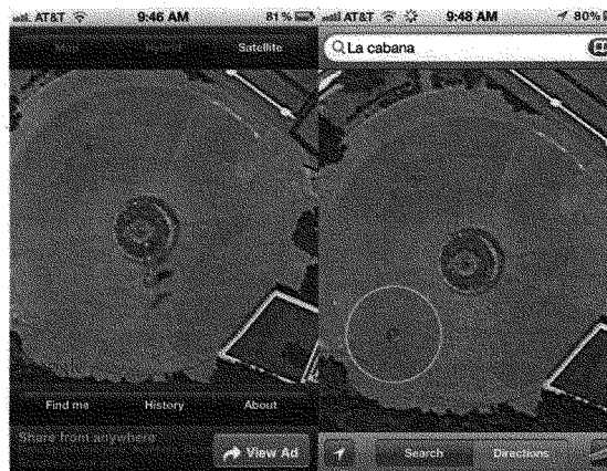
Fig. 13. (left) Corrected GPS position using GAIM-GM and SpoT-On concept (green dot is final position 2 m from center of traffic circle flower garden and (right) uncorrected position (blue dot) using an iPhone native GPS location.
