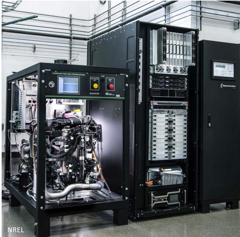
Leverage performance and economics of automotive fuel cell technology advances for new applications like a carbon-free data center with distribution fuel cell IT power.
