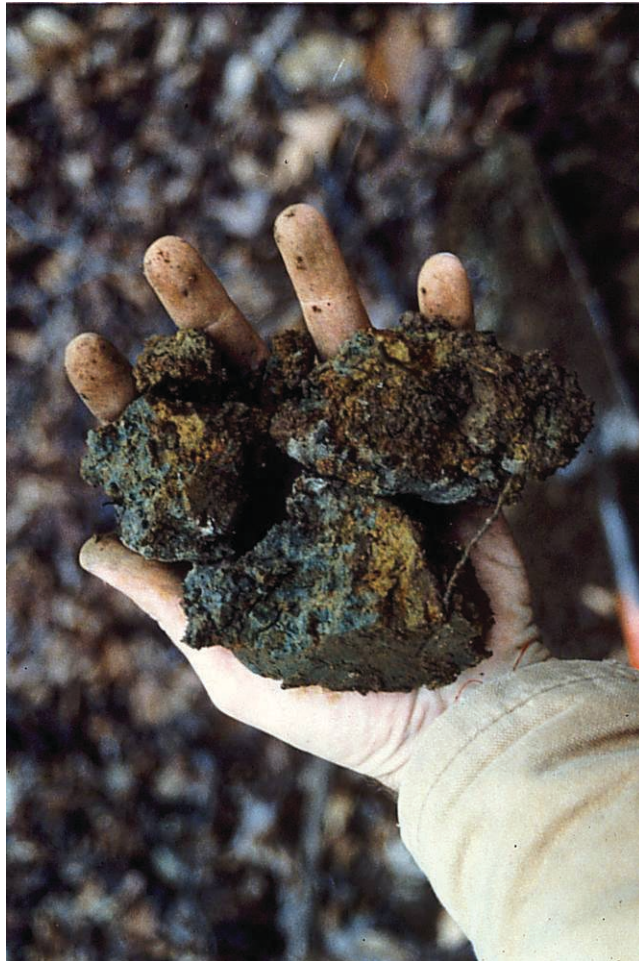
Figure 49.—Glaucanitic soils typically have gleyed, green, or black matrices and can have mottles of weathered sulfides that can be mistaken for redox concentrations. If the weathered sulfides in this glauconitic soil were mistaken for redox concentrations, this nonhydric soil would appear to meet the requirements of indicator F6 (Redox Dark Surface).
