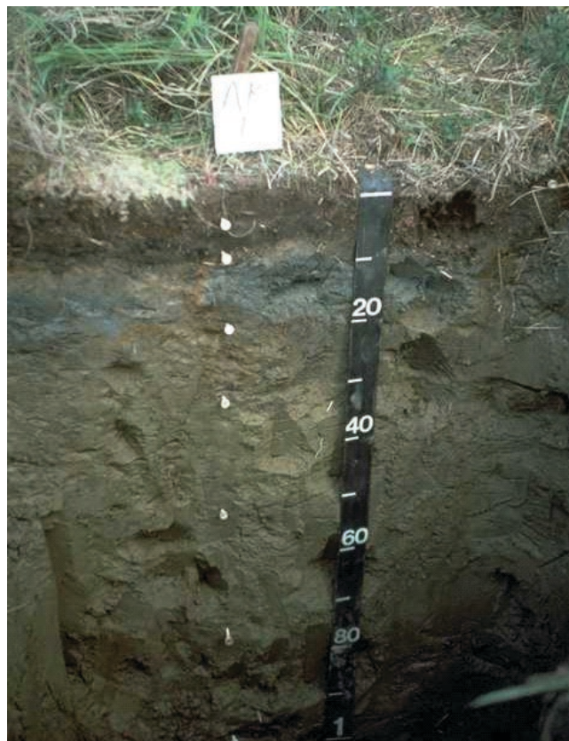
Figure 18.—Indicator A13 (Alaska Gleyed). The bluish band at a depth of about 20 cm indicates the presence of reduced soil material. The material below 20 cm reflects both the color of the parent material and soil weathering under aerobic conditions.
