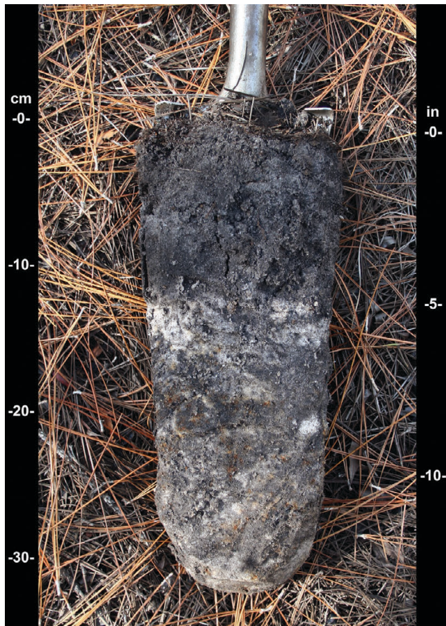
Figure 26.—Indicator S8 (Polyvalue Below Surface). The diffuse splotchy pattern of black (value of 3 or less and chroma of 1 or less) and gray (value of 4 or more and chroma of 1 or less) below a black surface horizon is evidence of organic matter that has been mobilized and translocated. This soil also meets the requirements of indicator S5 (Sandy Redox).
