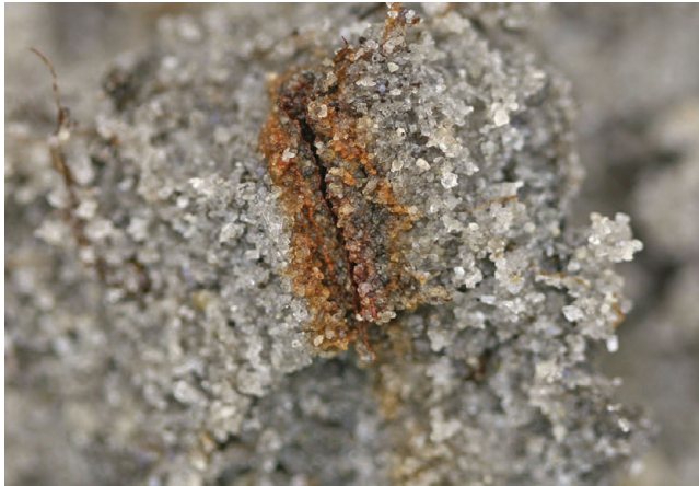
Figure 54.—A redox concentration occurring as a pore lining.
