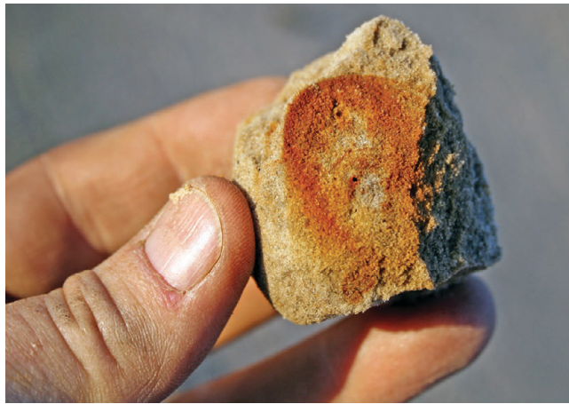
Figure 46.—Iron concentration with a diffuse boundary exhibited by bright colors in the center of the concentration and a lighter color away from the center.
