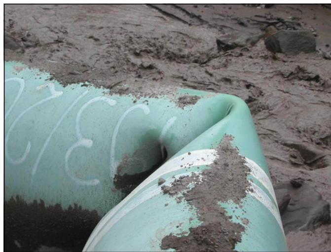
Figure 21. Photograph of an underground pipeline (buried 12 feet deep) that was excavated and crushed by a lahar during the 2002 eruption of Reventador volcano in Ecuador. Photograph by P. Ramon, Instituto Geofísico, Ecuador.
