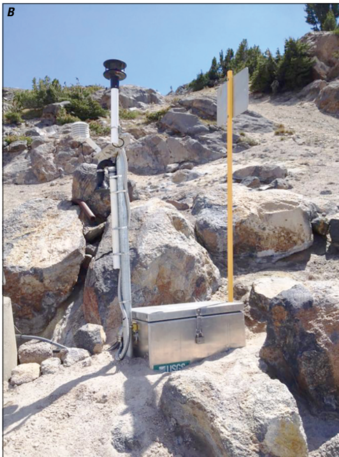
Figure 2. Photographs of volcano-monitoring sensors in the Long Valley volcanic region. Each sensor sends real-time data to scientists at the U.S. Geological Survey (USGS) California Volcano Observatory (CalVO). A , Global Positioning System (GPS) receiver for ground deformation monitoring (left) colocated with a seismometer (right). Photograph by S. Wilkinson, USGS. B , Sensors that monitor volcanic gas emissions. Photograph by P. Kelly, USGS.
