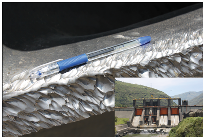
Figure 18. Photograph of a turbine at the Agoyan hydroelectric plant abraded by ash and other volcanic debris produced during eruptions of Tungurahua volcano, Ecuador. Inset photograph shows orange floodgates used to divert turbid water away from intake mechanisms. Photograph by J. Wardman, University of Canterbury.
