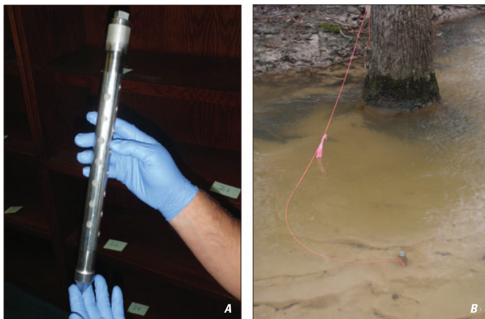
Figure 4. Drivepoint sampler (A) prior to being installed, and (B) installed in the hyporheic zone.
