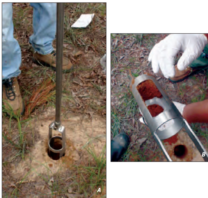
Figure 7. Soil sample (A) extracted with stainless-steel auger, and (B) transferred to sample container.
