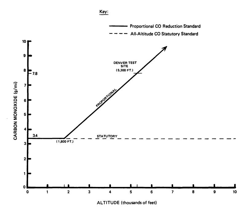
proportional standard for altitudes above 5,300 feet is found by extending the line to the desired elevation.
