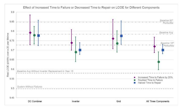
Fig. 3. Effect on LCOE of increased time to failure or decreased time to repair for the DC combiner, Inverter, Grid, or all three components combined, with baseline scenario lines for reference
