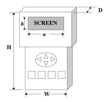
Figure #5: Diagram of scan tool measurements.
