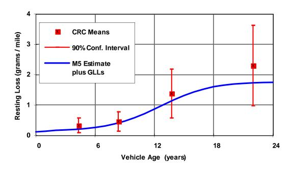
A visual examination of Figure 2 (or of Tables 2 and 3) indicates that for vehicles up through the age of 11 years, the re-weighted MOBILE5 predictions are excellent estimates of the mean CRC results (i.e., within 0.15 grams per mile). And, even
