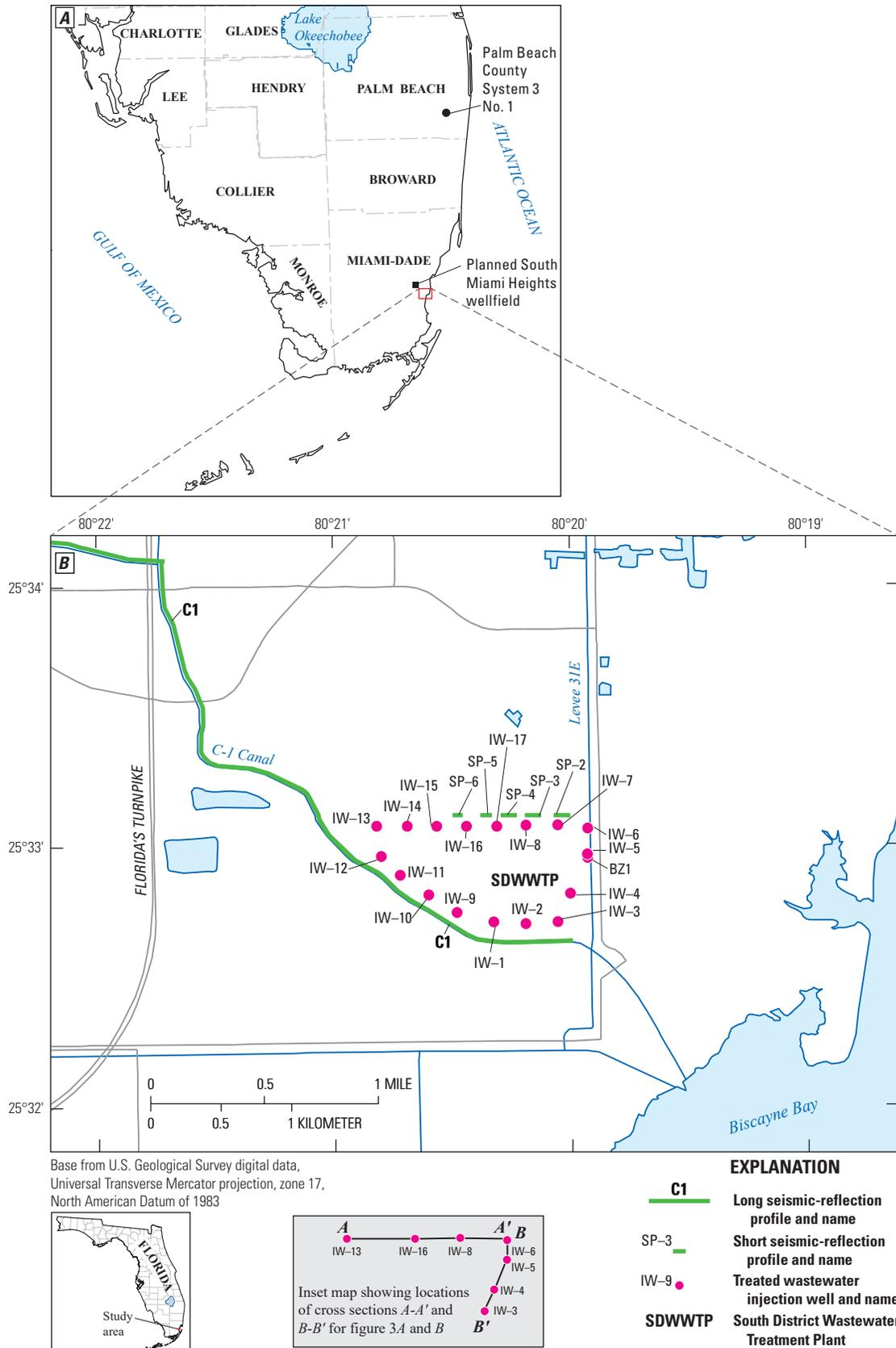
**Figure 1.** South District Wastewater Treatment Plant where injection wells IW-1 through IW-17 and monitor well BZ-1 are located and the location of seismic-reflection survey profiles in the study area (modified from Cunningham, 2015).
