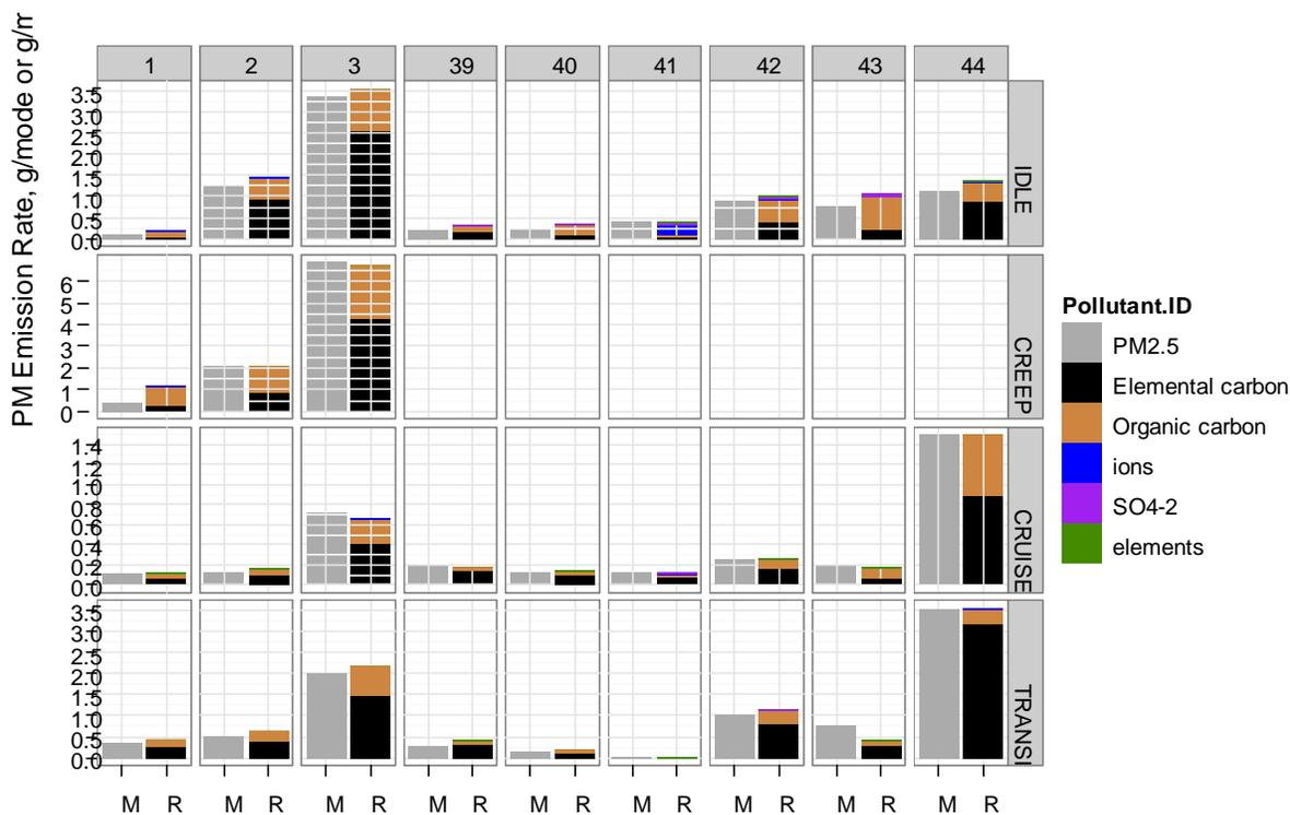
**Figure C-1. Average PM<sub>2.5</sub> Speciation Profiles by Truck and Test Cycle from the E55/59 Program. M = Measured total PM<sub>2.5</sub>, R = Reconstructed total PM<sub>2.5</sub> from the speciated measurements**
