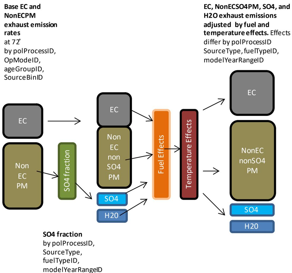
Figure 2. Flow Chart of Calculation of the Intermediate PM<sub>2.5</sub> Emission Rates
