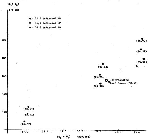
\*The values in parenthesis under each point are the rear roll velocities in (MPH)
