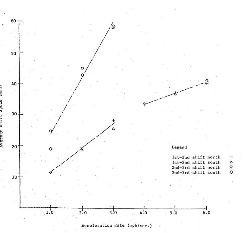
in lst-2nd gear shift speed at an acceleration rate of 4 mph/sec than anticipated from the shift points at the first three acceleration rates. Vehicle B experienced less of a dramatic change of lst-2nd gear shift speed between the acceleration rates of 3 to 4 mph/sec.
