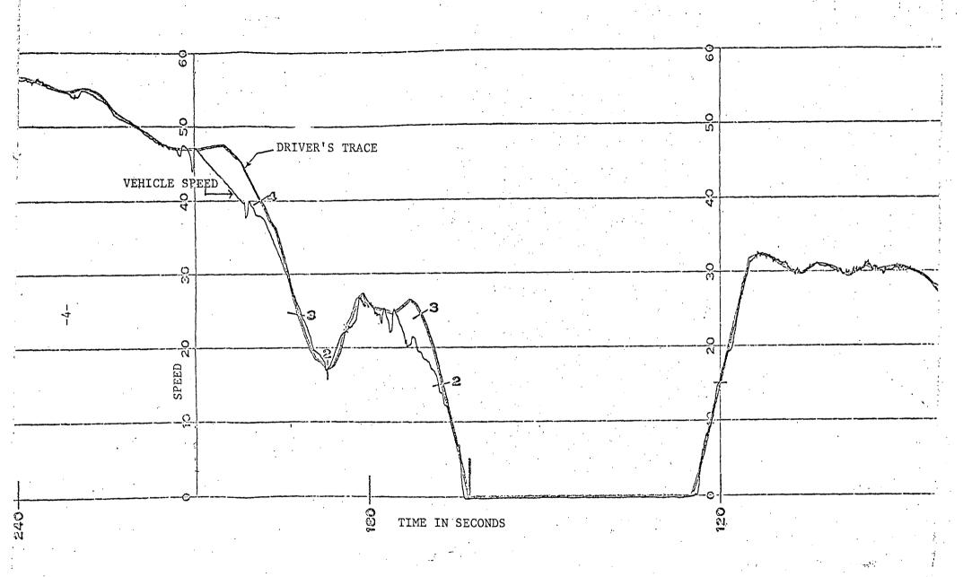
FEDERAL DRIVING SCHEDULE VOLUME 36 NUMBER 55 MARCH 20, 1971 (Driving Trace from Test 16-491, Shifting at 3500 RPM Engine Speed)
