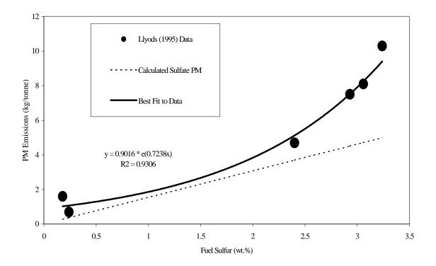
Figure 1-1. Effect of fuel sulfur on particulate emissions rates.
