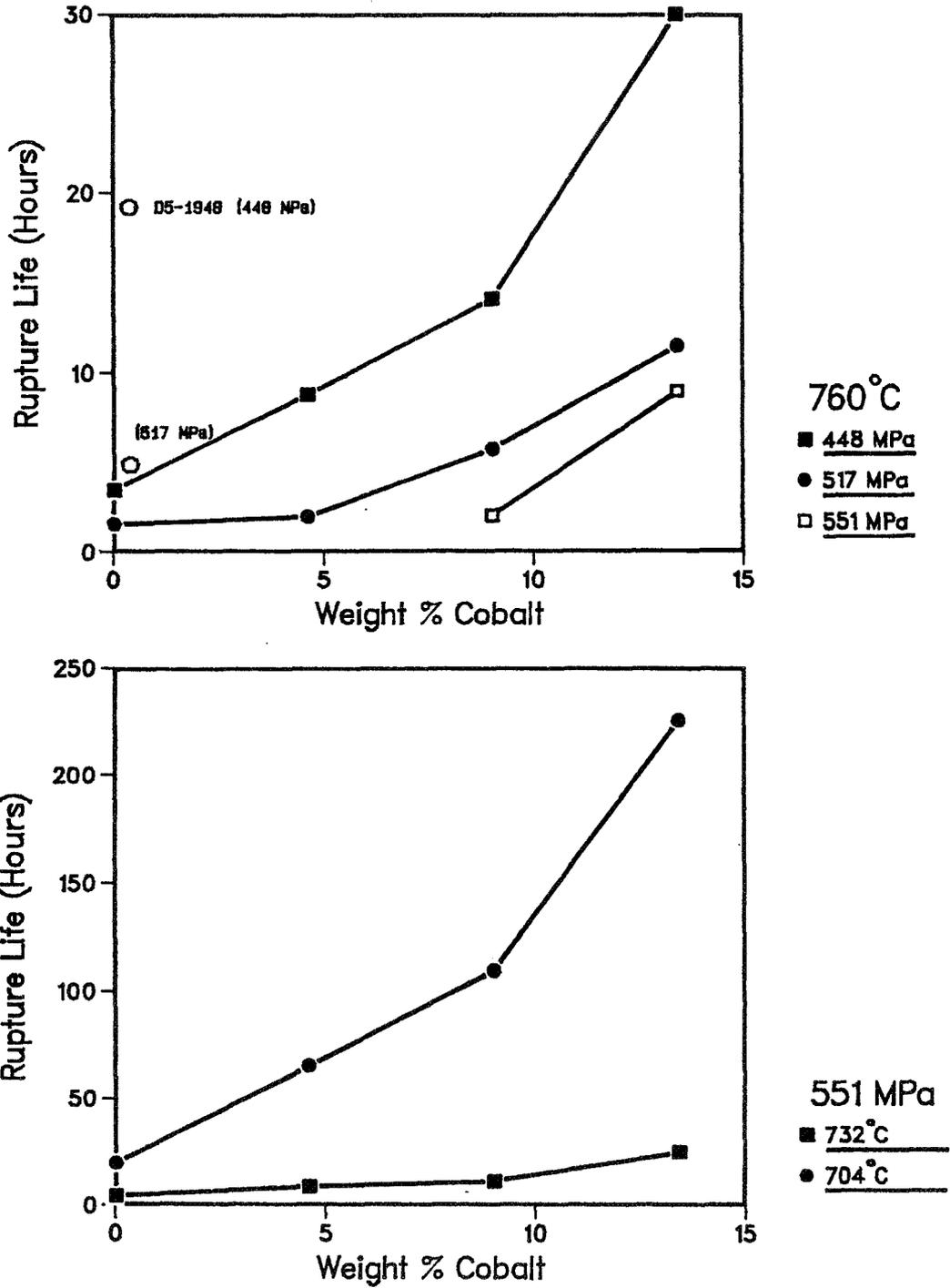
Figure 3. Stress rupture lives of Waspaloy as a function of cobalt.
