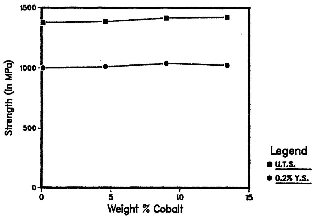
Figure 2. Tensile strength of Waspaloy as a function of cobalt.
