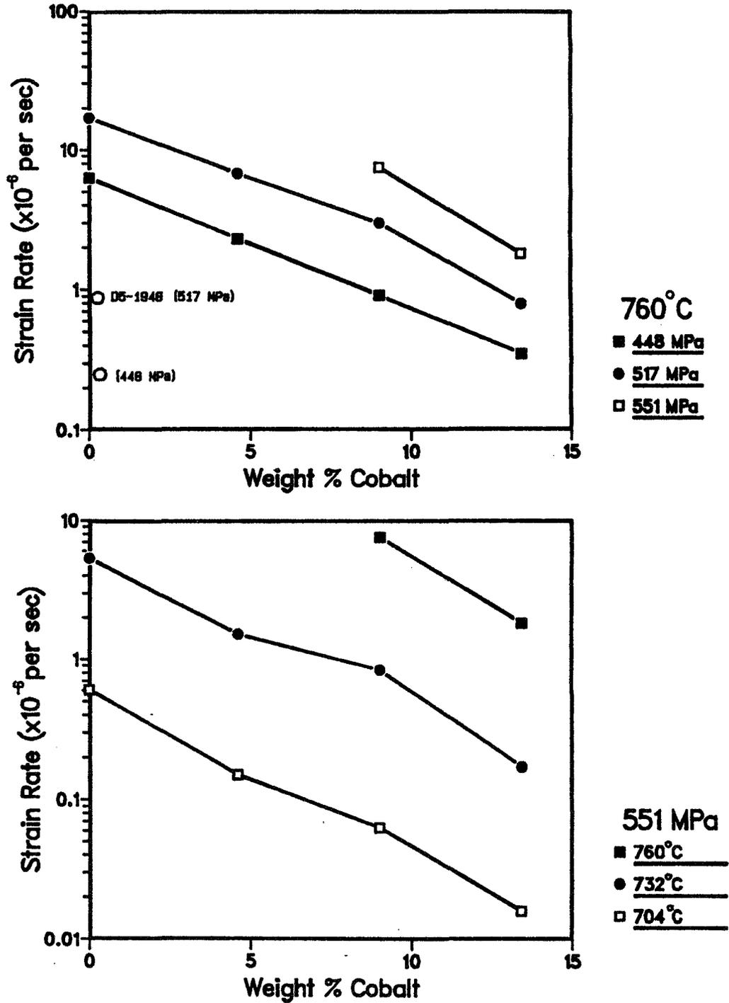
Figure 4. Minimum creep rates as a function of cobalt content. Note that the cobalt free alloy with additional (Al+Ti) shows the same creep rate as the alloy with the standard cobalt, aluminum and titanium contents.
