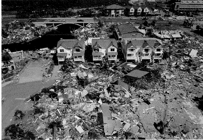
Figure 3: Mexico Beach, FL after Hurricane Michael (2018). Older homes not built to code are completely destroyed. But newer homes built to code suffered relatively minor damage. (Dronebase/Reuters, Handout/Reuters).
