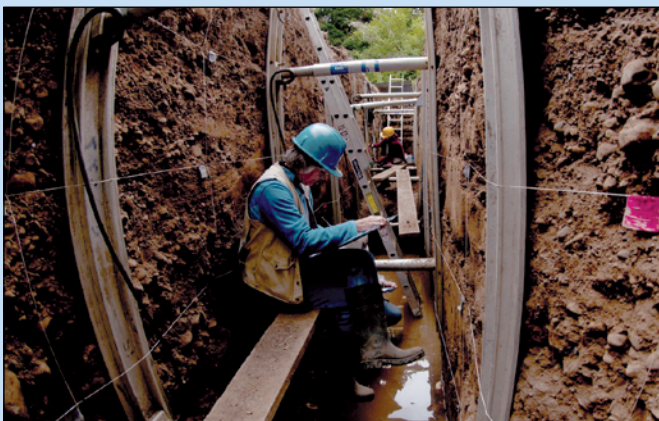
To assess the recurrence interval of major earthquakes on the San Andreas Fault, Earthquake Science Center scientists dug a trench across the fault to study the offset and age of soils that have been disrupted by prehistoric earthquakes.
