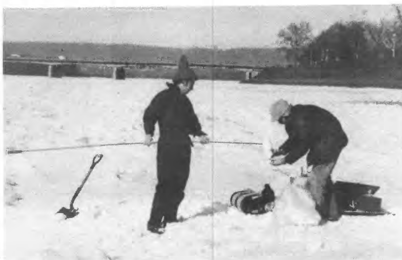
Figure 9.--Depth-integrated sampling just upstream from Walnut Street Bridge during period of full ice cover on January 19, 1981.
