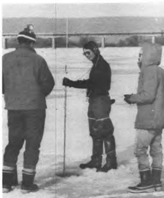
Figure 7.--Streamflow measurement on January 19, 1981 when ice covered entire channel of Susquehanna River at Harrisburg.
