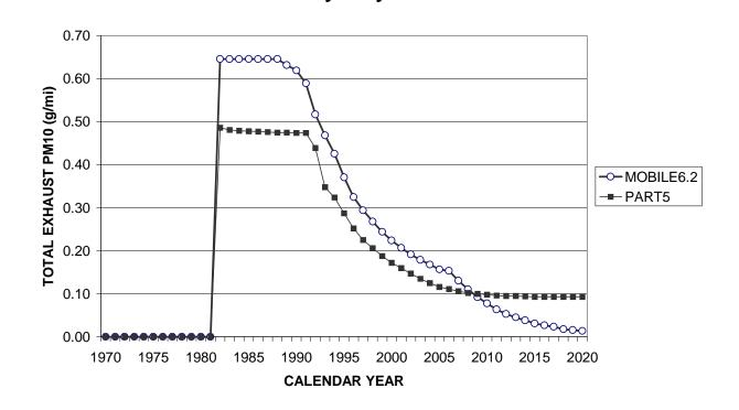
MOBILE6.1 and PART5 Total Exhaust PM10 Emissions from Medium Heavy-Duty Diesel Vehicles
