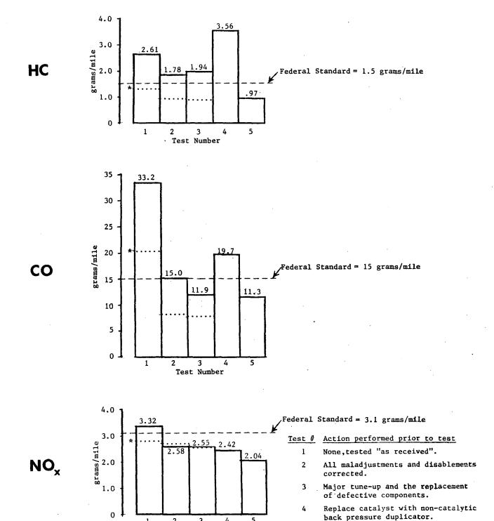
\*Note: Dotted lines represent fleet average emissions of 300 1975 and 1976 Restorative Maintenance Vehicles tested in a earlier program (Reference 1).
