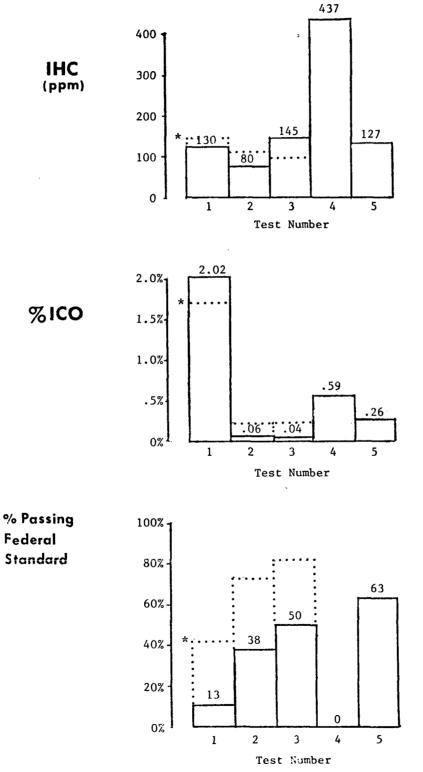
\*Note: Dotted lines represent fleet average emissions of 300 1975 and 1976 Restorative Maintenance Vehicles tested in a earlier program (Reference 1).
