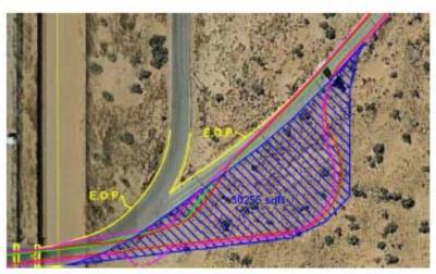
Figure 2. Curved lane. - Tip Swing. - Truck Front Axel. - Back Axel
