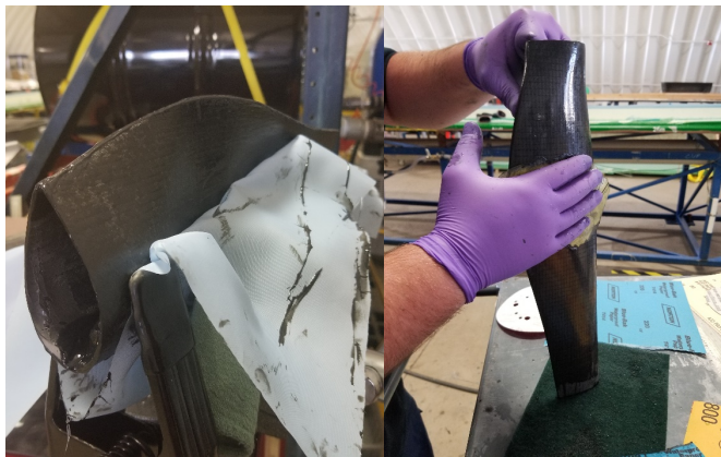
Fig. 10. (left) adhesive bonding process; (right) wet sanding and surface preparation
