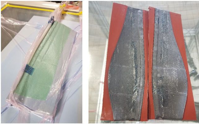
Fig. 9. (left) infusion process; (right) blade skins in mold after infusion
