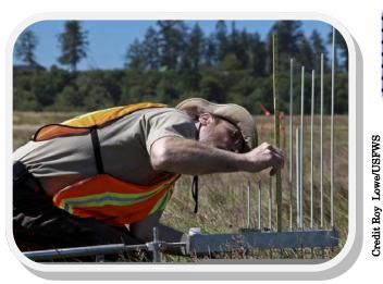
USFWS biologist Bill Bridgeland taking measurements which will allow the Service to detect changes in marsh surface elevation from restoration efforts and changes associated with sea-level rise.
