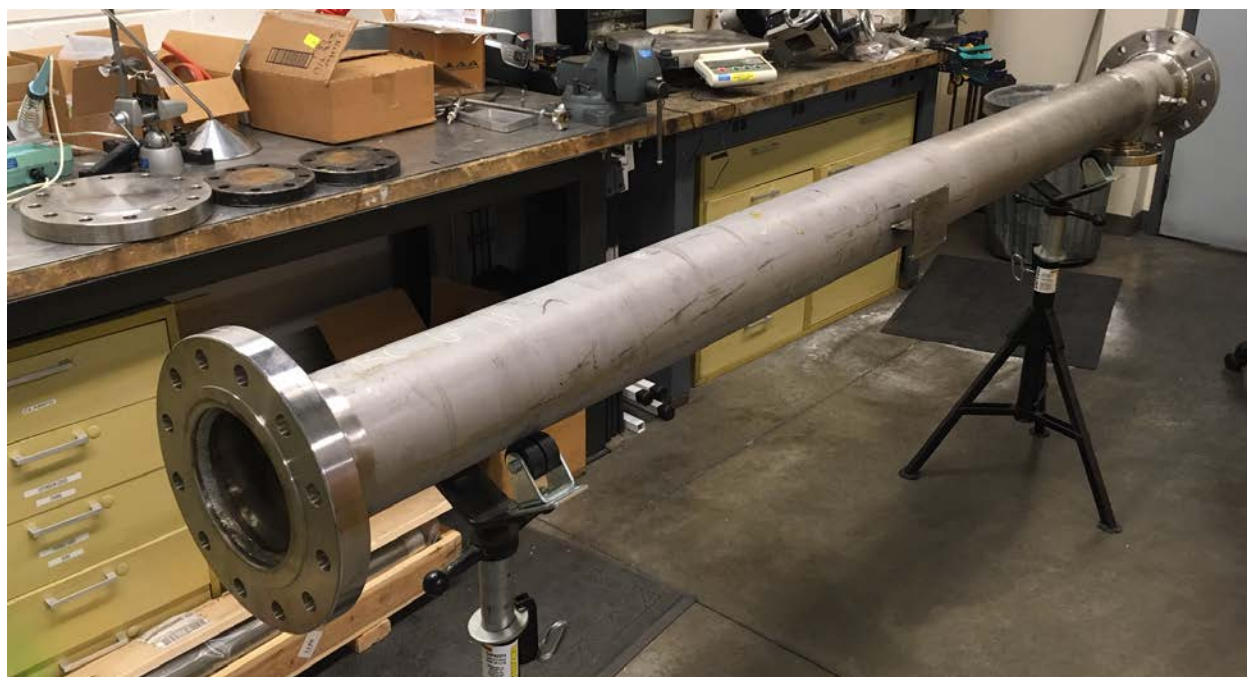
Figure 51. Integrated hydrogen sensor/separation module.
