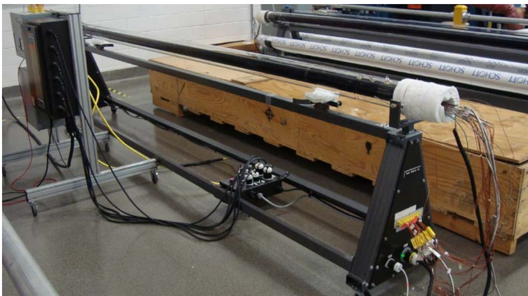
Figure 16. NREL heat-loss test stand for daily heating of in-service receiver.
